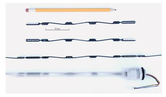
**Figure 4.** Modular design of the sensor probe. From top to bottom: top view of a sensor board, bottom view of a sensor board, cascaded sensor boards, and final probe assembly containing an array of cascaded sensor sections in a 3/8 in. ( $\sim$ 10 mm) outer diameter tube, filled with epoxy.
