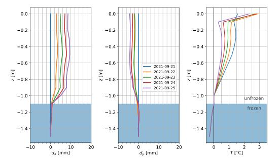
**Figure 14.** Field measurements obtained over five days at a field site on the Seward Peninsula, AK which is experiencing soil movements in response to permafrost thaw. Left and middle panels show the displacement along the *x* and *y*-axis, respectively; right column shows the soil temperature. Highlighted in blue is the frozen part of the subsurface, showing that the slip plane is colocated with the interface between frozen and unfrozen soil.
