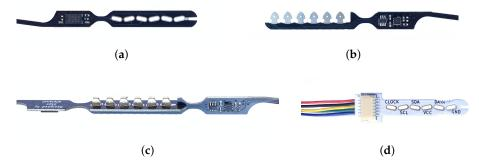
**Figure 3.** Close-ups of the proposed connector technology. (a) Female connector piece; (b) Male connector piece; (c) Mated connector; (d) Wire-to-Board adapter.
