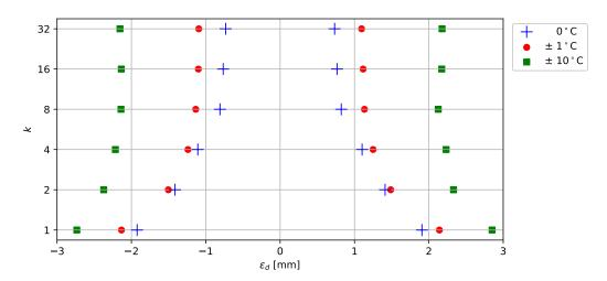
**Figure 13.** Deformation error ( $\epsilon_d$ ) in function of number of averaged measurements (*k*) expressed as 2.5th and 97.5th percentiles for 0 °C,  $\pm$ 1 °C and  $\pm$ 10 °C temperature variations.
