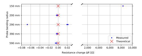
Figure 11. Trace resistance under bending.
