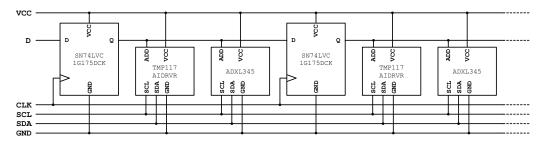
Figure 2. Schematic of cascaded temperature sensors and accelerometers in a shift register configuration
