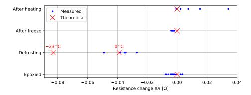
Figure 10. Trace resistance under freezing, heating, and epoxying.
