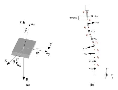
**Figure 1.** Accelerometer arrays can be used for deformation measurements. (a) Inclination measurement with an accelerometer and (b) design of the probe with temperature sensors  $(T_i)$  and accelerometers  $(\mathbf{a}_i)$ .
