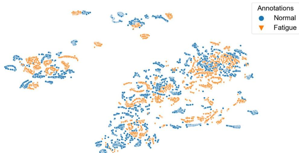
**Figure 13.** t-SNE visualization illustrating the low-dimensional signal distribution of all datasets from the muscle fatigue study two, color-coded according to the muscle state (normal vs. fatigue). The t-SNE parameters were set to a perplexity of 200, a learning rate of 200, and 10,000 iterations.
