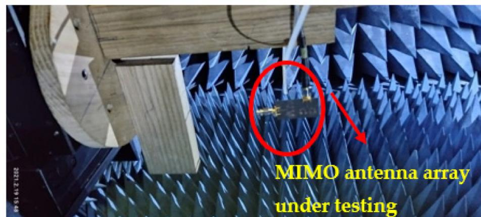
Figure 6. Proposed MIMO antenna array under testing.
