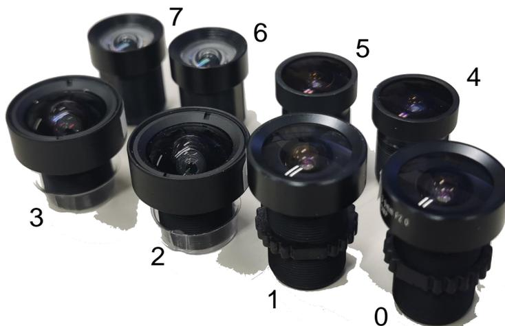
**Figure 7.** An illustration of the eight lenses that were used in our experiments. Lenses 0 to 3 are high resolution, while Lenses 4 to 7 are low resolution. The imaging capability of Lens 0 is very inconsistent, while Lens 1, Lens 4 and Lens 5 are a little bit inconsistent and the remaining four lenses are good.
