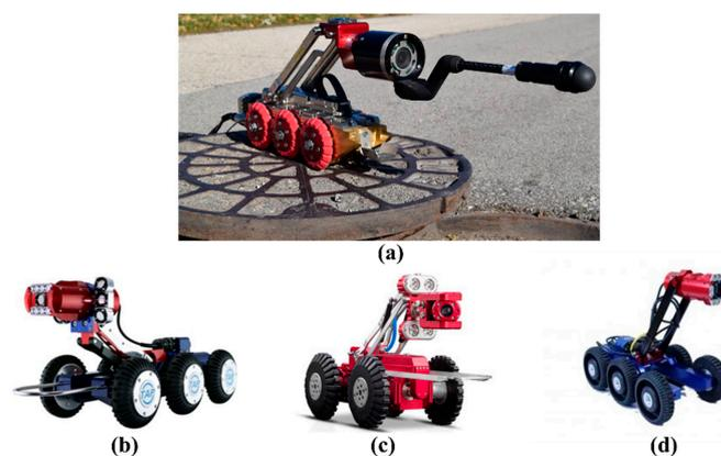
**Figure 12.** Representative inspection robots for data acquisition. (a) LETS 6.0, (b) Robocam 6, (c) X5-HS, and (d) Robocam 3000.
