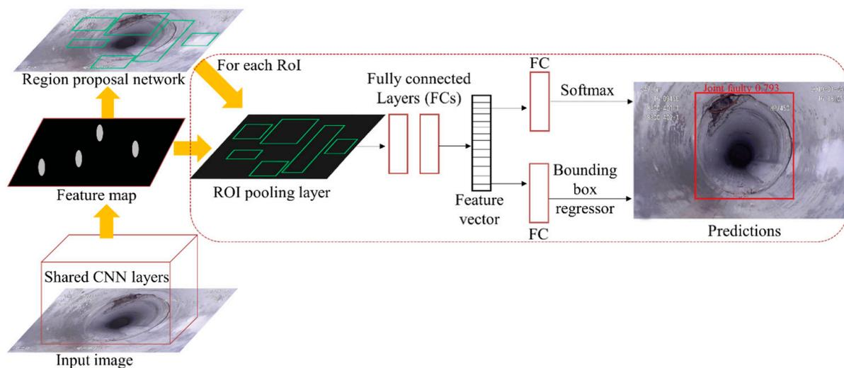
**Figure 10.** An architecture of the faster R-CNN developed for defect detection. ‘CNN’ refers to convolutional neural network. ‘ROI’ means region of interest. ‘FC’ is fully connected layer.
