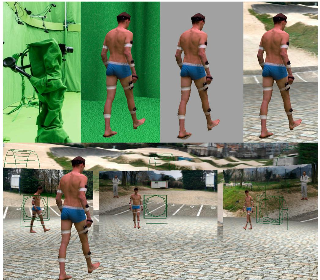
**Figure 2.** Participant's 3D textured meshes were extracted using 68 video cameras in the studio, and then placed in a virtual environment. The scene was then filmed from 8 virtual cameras.
