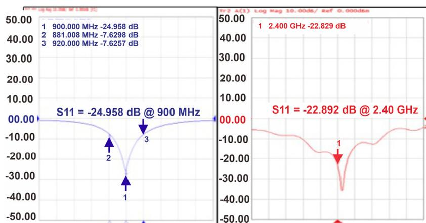
**Figure 6.** Measured  $|S_{11}|$  for the RF-DC converter at a  $1\text{ M}\Omega$  load.
