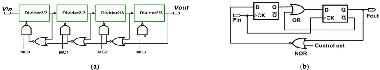
Figure 7. The proposed (a) Multiple modulus divider circuit; and (b) the 2/3 divider circuit.
