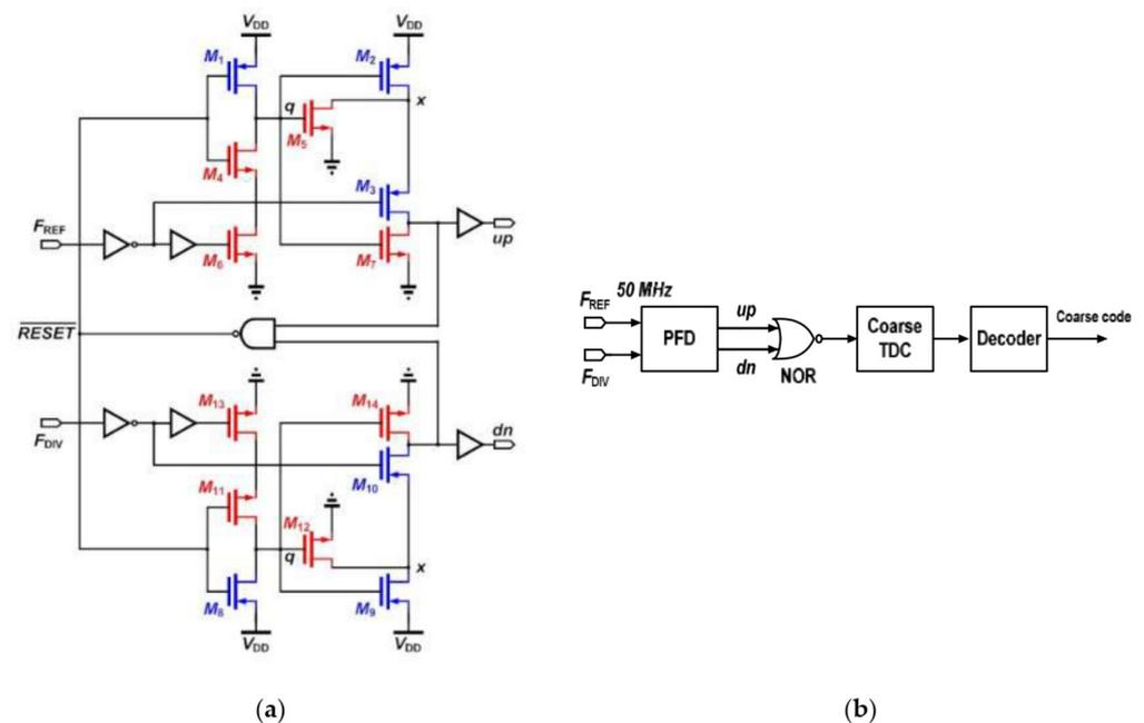
Figure 3. The proposed (a) frequency phase detector circuit; and (b) frequency detector structure.
