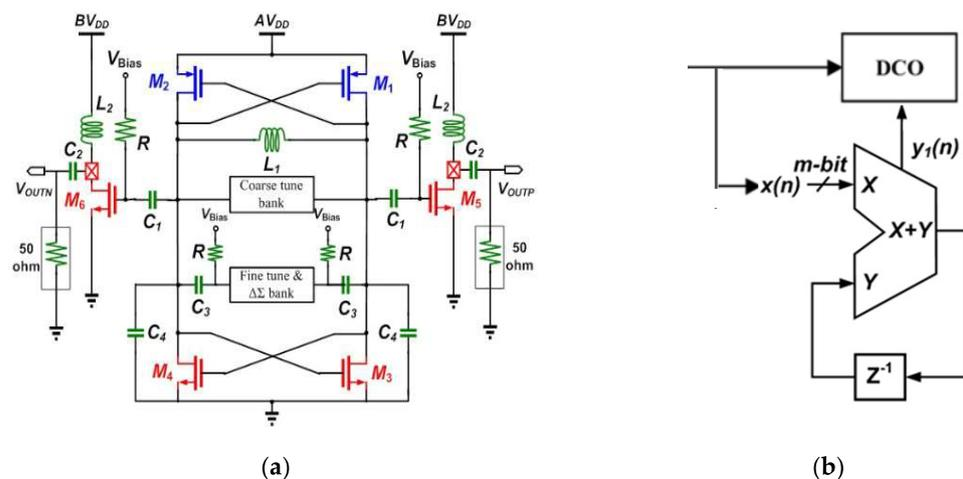
**Figure 2.** The proposed (a) LC-Tank VCO circuit; and (b) structure of the first-order delta-sigma modulator.
