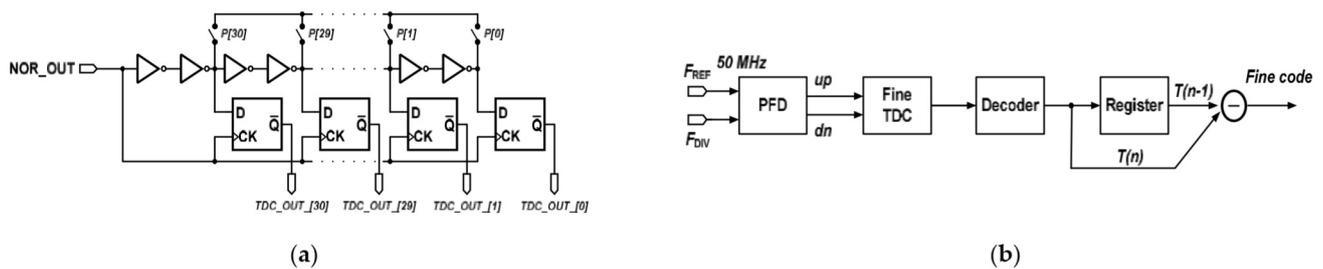
Figure 4. The proposed (a) coarse TDC structure using 31 stages; and (b) phase detector structure.
