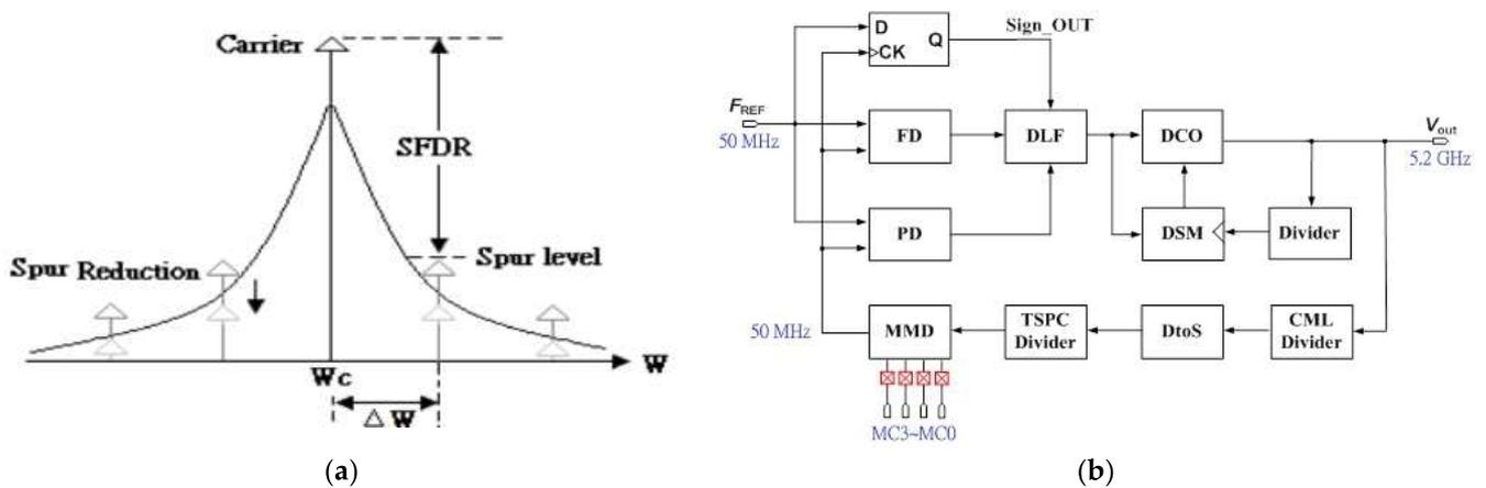
**Figure 1.** (a) Frequency domain representation of spurs; and (b) the function block of the introduced all-digital frequency synthesizer.
