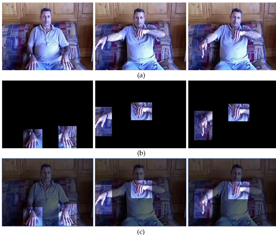
**Figure 2.** Sample of different data used in local attention: (a) raw RGB data; (b) hand data processed by hand detector; (c) fusion of raw RGB data and hand data.
