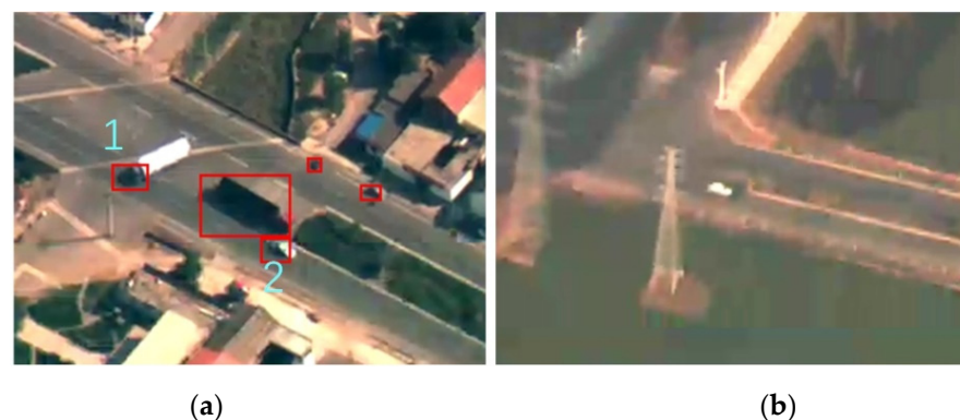
Figure 3. Example of missed white vehicles. Detection boxes 1 and 2 in (a) only detect the black cabin of the white truck or the black shadow around the white vehicle, while ignoring the real objects. (b) demonstrates that the only white object is not detected.
