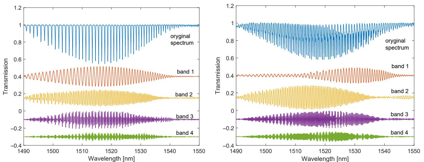
**Figure 9.** Optical spectra: original and band-filtered for individual frequency ranges for the TFBG and DC-TFBG (SRI = 1.333).
