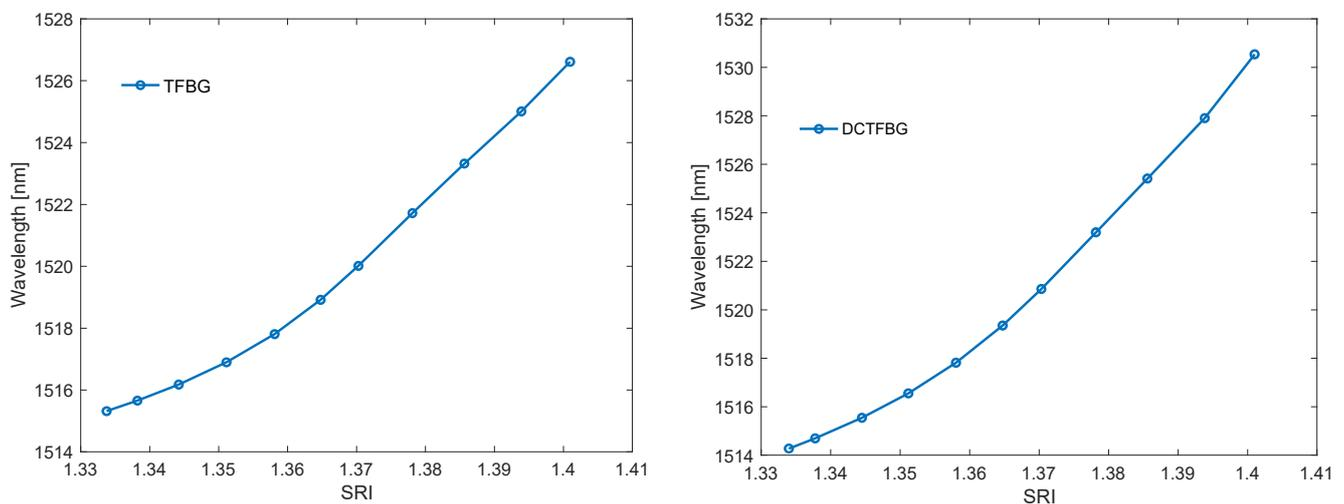
**Figure 15.** Change in the wavelength of the centre of gravity of the TFBG optical spectrum after band filtration for band 1 and for DCTFBG for band 2 filtration.
