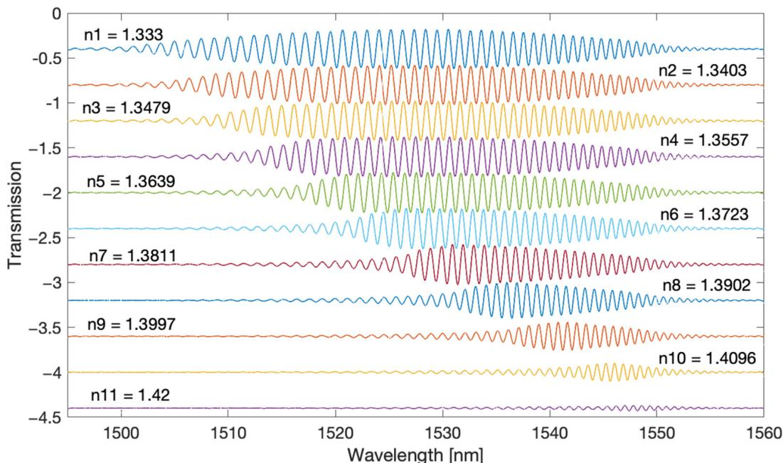
Figure 4. TFBG spectra after Fourier filtering for the first (main) frequency band.
