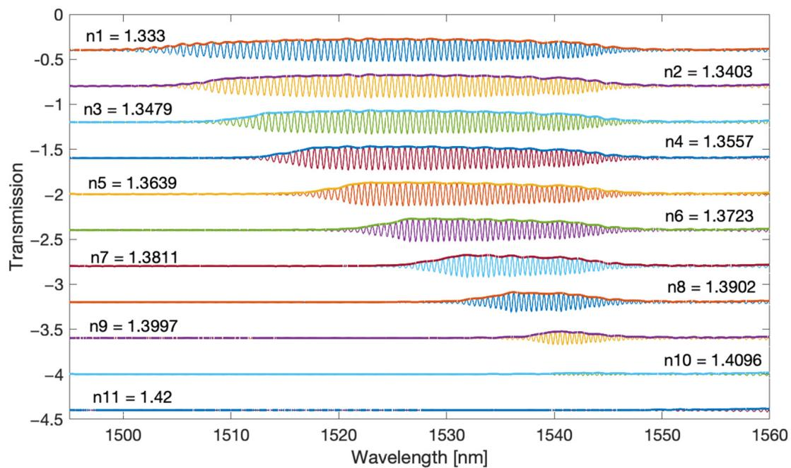
Figure 7. Envelope calculated by the Hilbert transform method for the second frequency band.
