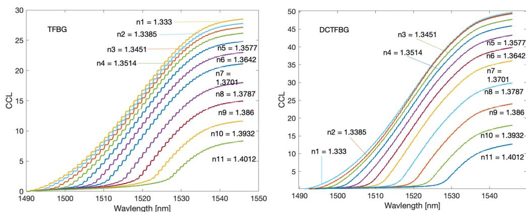
**Figure 16.** Cumulative spectrum contour for TFBG and DC-TFBG.
