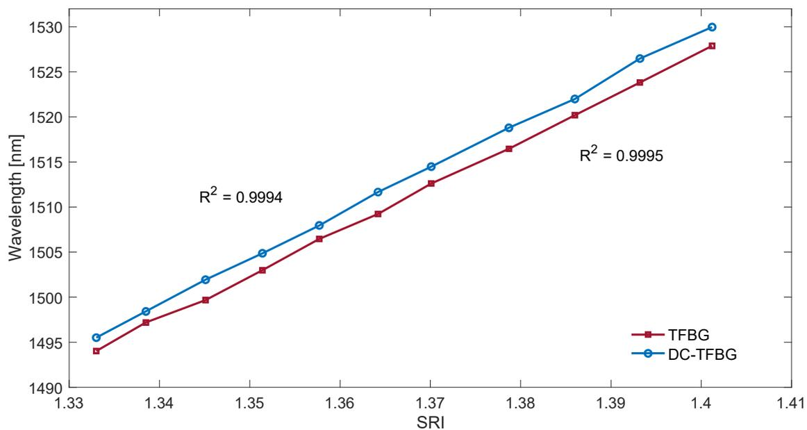
**Figure 18.** The wavelength of the second derivative maximum of the cumulative contour spectrum for TFBG and DCTFBG.
