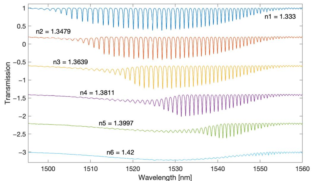
**Figure 2.** Optical spectrum of the TFBB for several SRI values.
