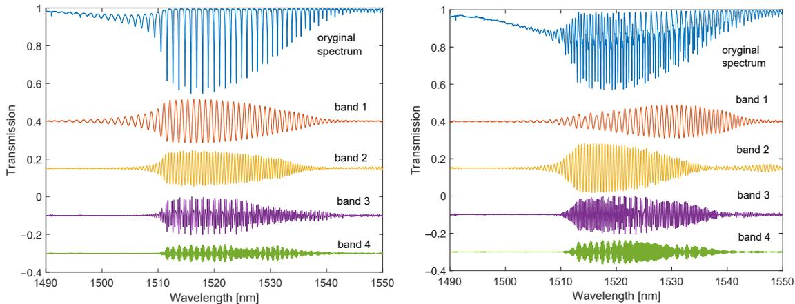
Figure 10. Optical spectra: original and filtered for individual frequency bands for TFBG and DC-TFBG (SRI = 1.3701).
