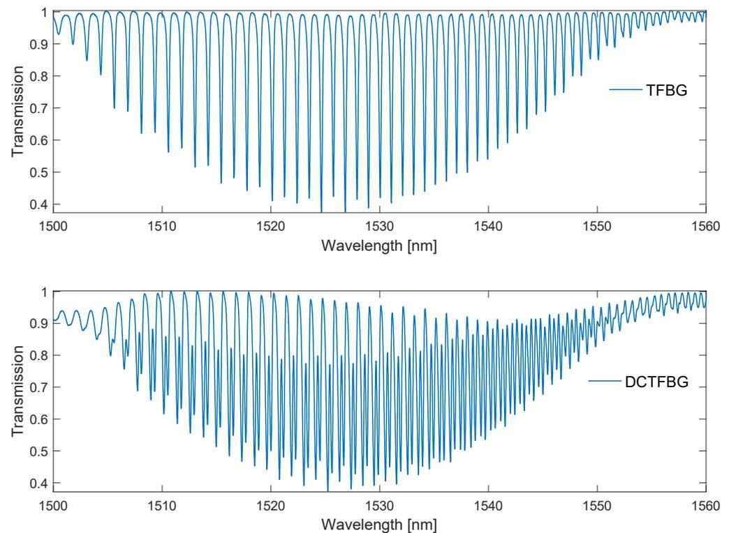
**Figure 1.** Spectrum of a TFBG and of a DC-TFBG, the latter being one of the gratings produced by us.
