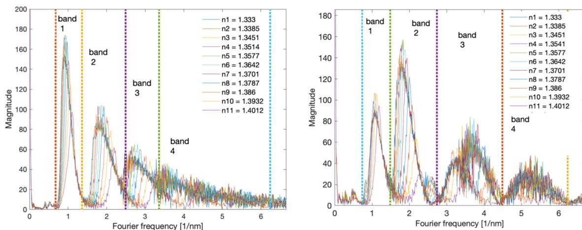
Figure 8. Comparison of Fourier spectra of TFBG and DC-TFBG gratings for individual SRI values.
