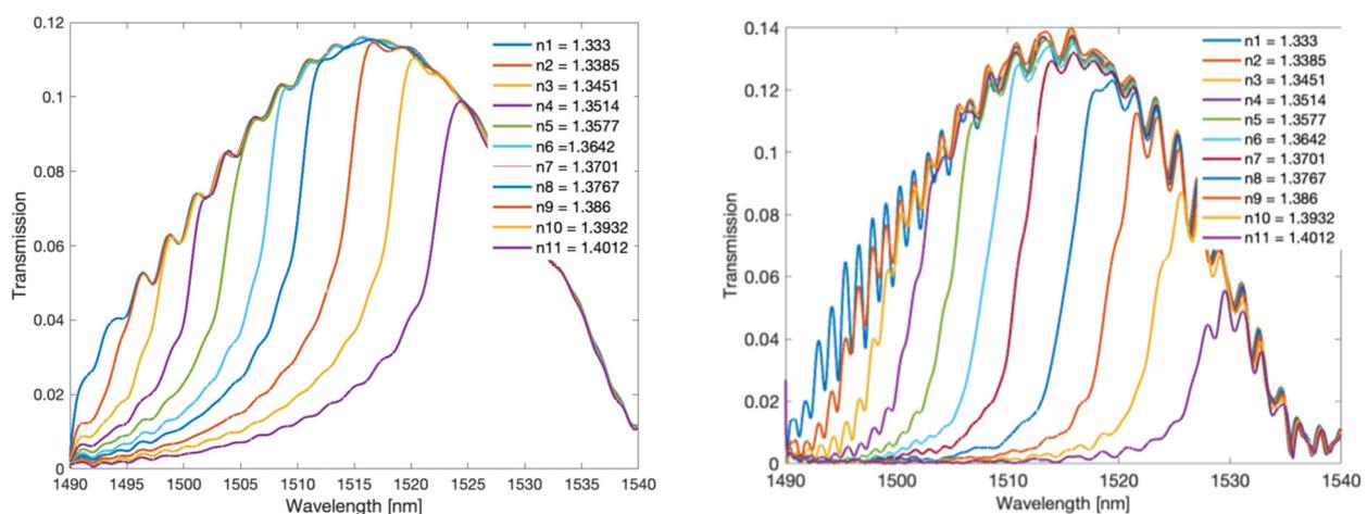
**Figure 13.** Changing the spectrum of the Hilbert envelope from SRI for band 1 of the TFBG and band 2 for the TCTFBG.
