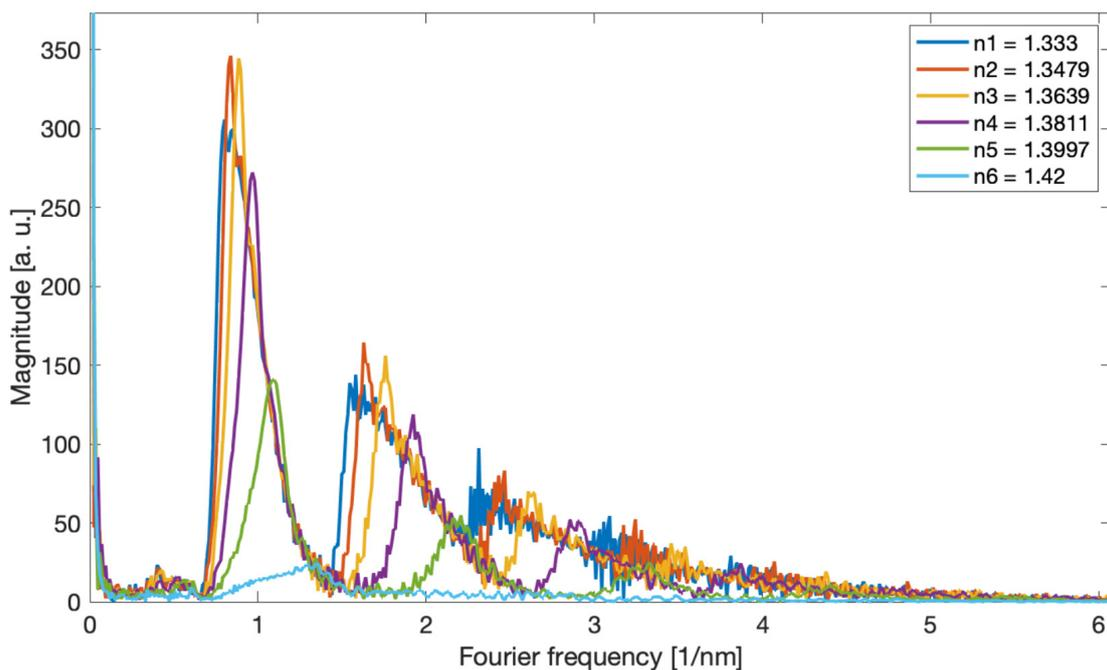
Figure 3. The amplitude Fourier spectrum corresponding to the optical spectra of the TFBG in Figure 2, depending on the SRI.
