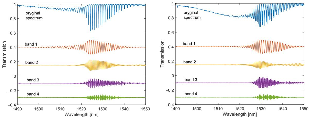
Figure 11. Optical spectra: original and band-filtered for individual frequency bands for TFBG and DC-TFBG (SRI = 1.4012).
