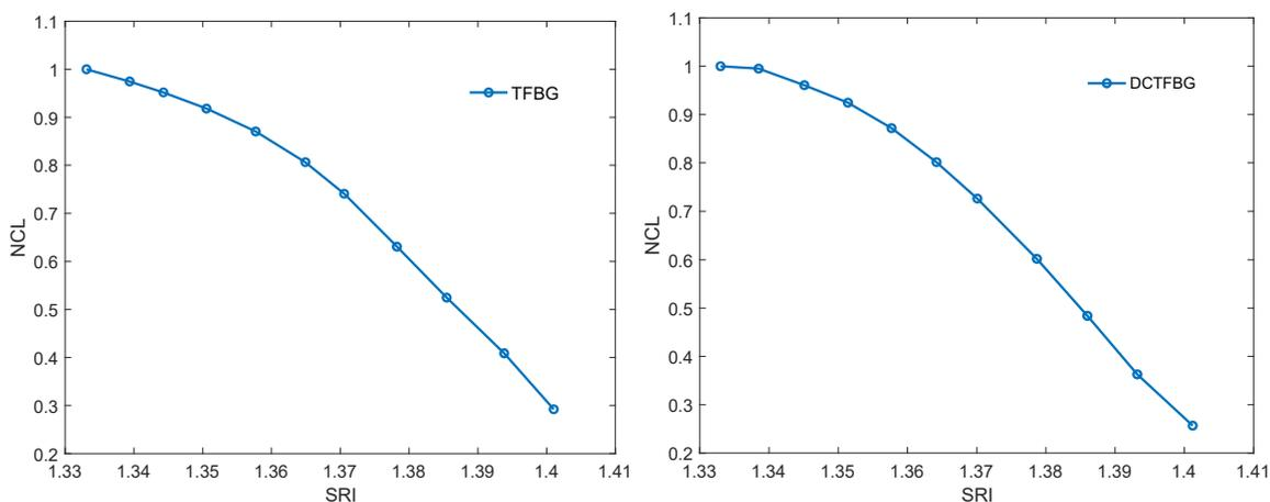
Figure 12. Change of the normalised contour length from SRI for the TFBG and DC-TFBG.
