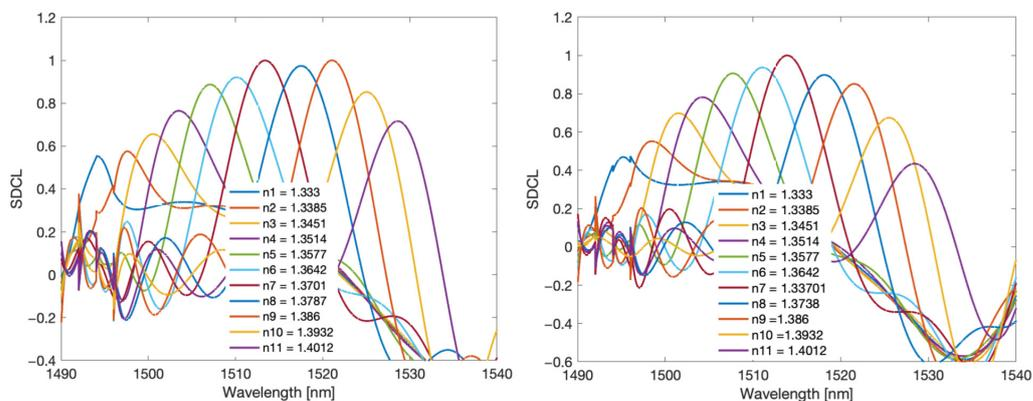
**Figure 17.** Second derivative of the cumulative spectrum contour for TFBG and DCTFBG.
