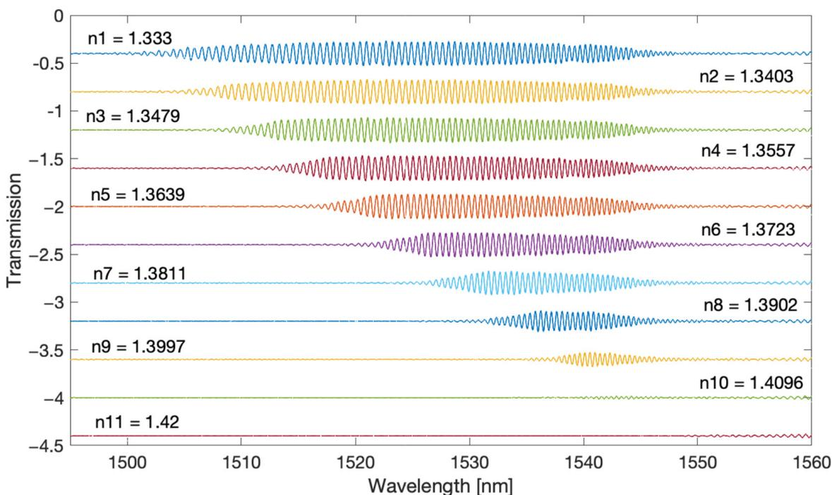
Figure 5. TFBG spectra after Fourier filtering for the second frequency band.
