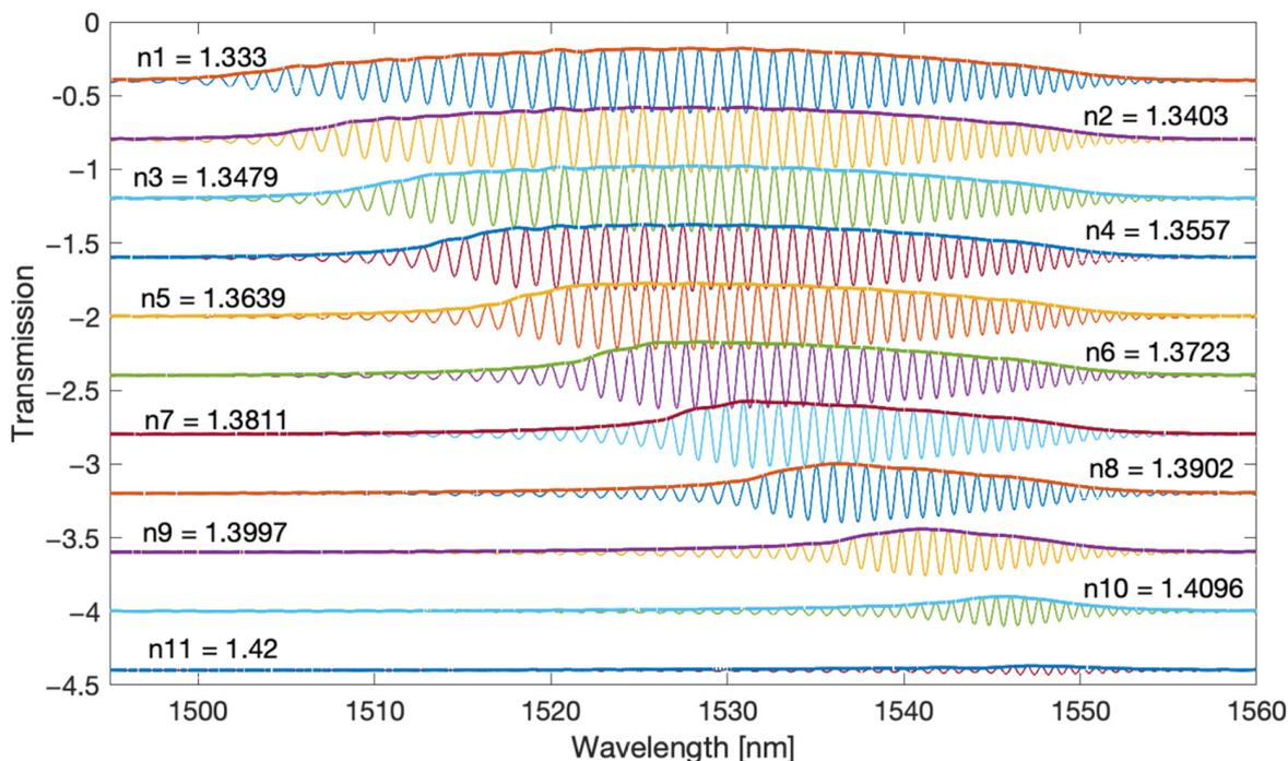
Figure 6. Envelope calculated by the Hilbert transform method for the main frequency band.
