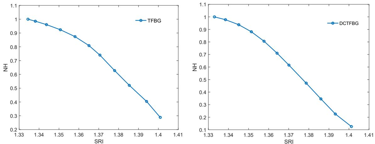
**Figure 14.** Change of normalised Hilbert envelope from SRI for TFBG (band 1) and DCTFBG (band 2).
