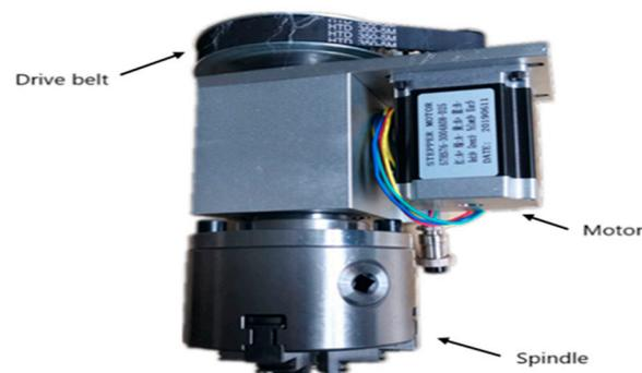
**Figure 1.** Rotary spindle unit of a CNC milling machine. (Source: <https://www.dec-motor.com/>, accessed date: 4 December 2021).
