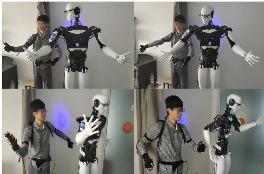
**Figure 12.** Experiments of different gestures with arms and head.
