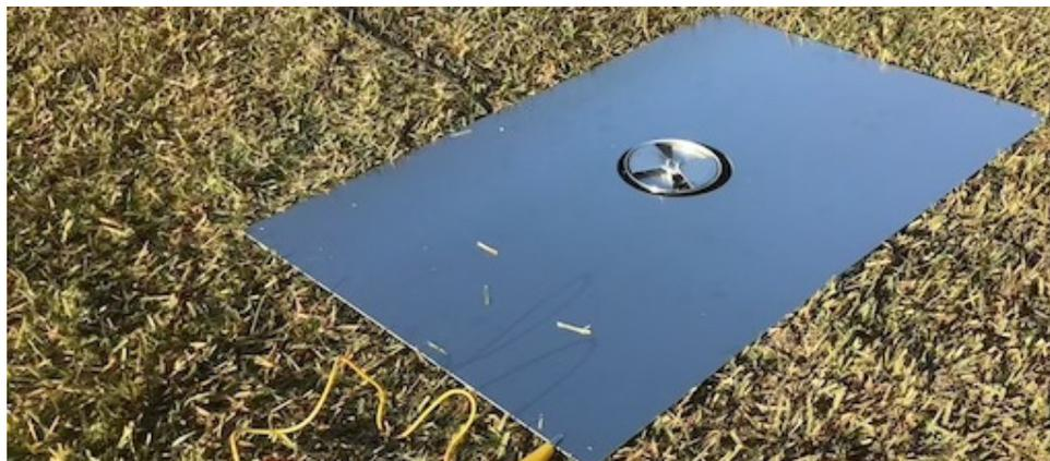
**Figure 4.** Picture of EFM system temporarily installed to measure the fair-weather electric field at ground level.
