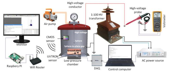
**Figure 3.** Experimental Setup. Diagram of the experimental setup including the instrumentation used for the detection of corona in the high-voltage tests with their respective diametric measures.
