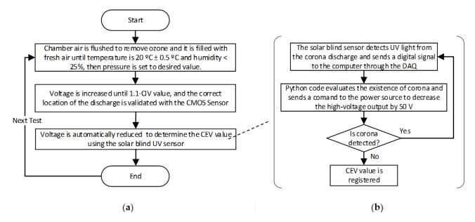
**Figure 1.** Procedure to determine the value of the CEV value of the sphere-to-plane air gaps. (a) Process overview. (b) Automatic acquisition of corona extinction voltage values using python process.
