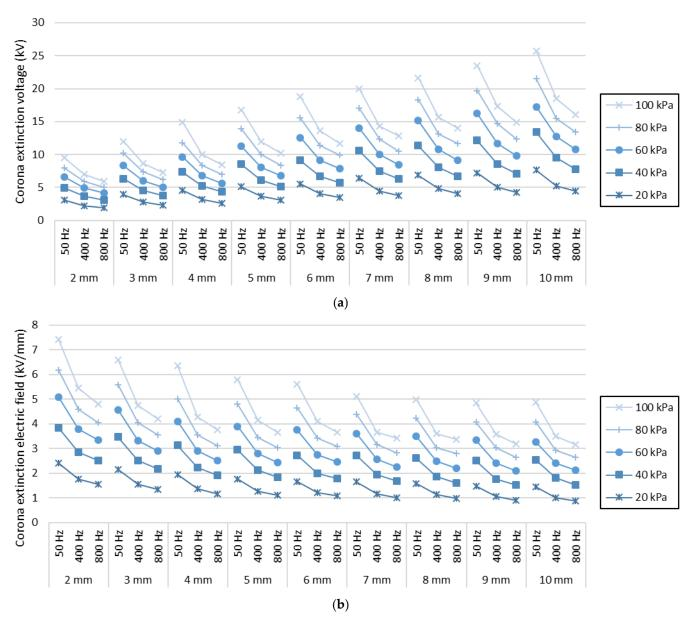
**Figure 5.** Visual representation of experimental values obtained from Table 1. (a) Corona extinction voltage. (b) Corona extinction electric field.
