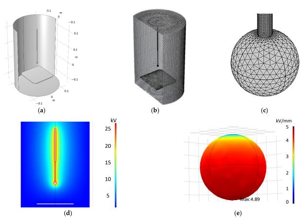
**Figure 2.** Simulation setup. (a) 3D geometry within the simulator. (b) Representation of the selected mesh. (c) Detail of the surface mesh on the sphere electrode. (d) Simulation of the electric potential around the electrode. (e) Simulation of the electric field on the sphere surface.
