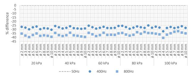
**Figure 8.** Corona extinction electric field strength (CEV conditions). Percentage difference at 400 Hz and 800 Hz referred to 50 Hz.
