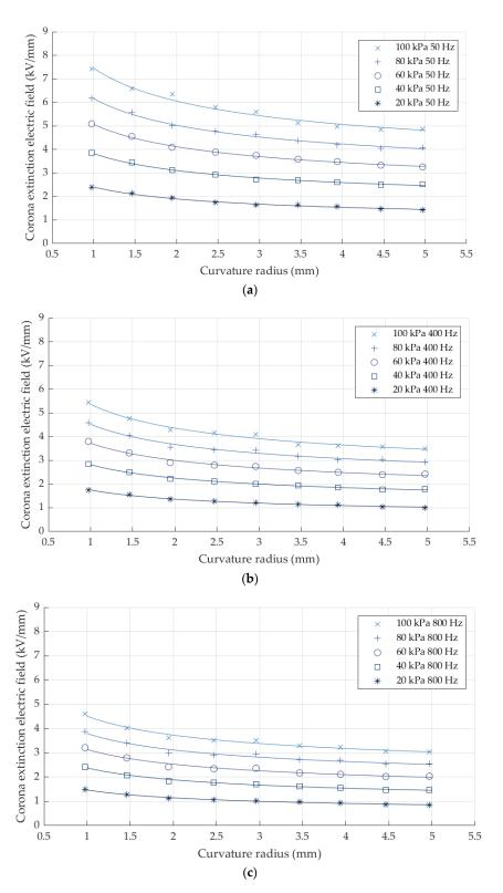
**Figure 6.** Corona extinction electric field strength versus the curvature radius of the sphere. (a) Peak's curve regression for 50 Hz. (b) Peak's curve regression for 400 Hz. (c) Peak's curve regression for 800 Hz.
