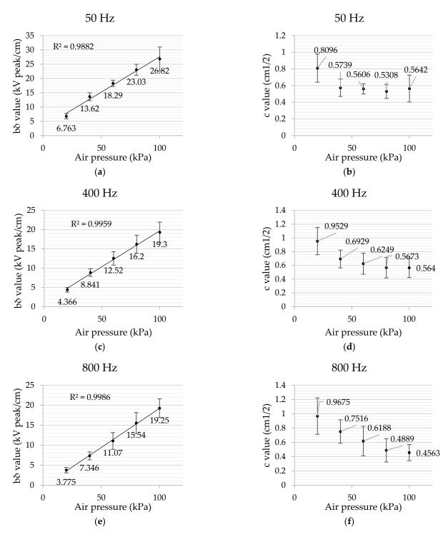
**Figure 7.** Coefficients  $b\delta$  and c resulting from the fitting of the experimental data to the generalized Peek's law with 95% confidence bounds. (a)  $b\delta$  coefficient values at 50 Hz. (b) c coefficient values at 50 Hz. (c)  $b\delta$  coefficient values at 400 Hz. (d) c coefficient values at 400 Hz. (e)  $b\delta$  coefficient values at 800 Hz.
