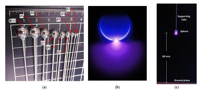
**Figure 4.** Sphere electrodes. (a) Photograph of the sphere electrodes used in the experiments. With the respective diameters. (b) Corona image taken with the CMOS imaging sensor to validate the location of the corona discharges before CEV acquisition. (c) Photograph of the sphere-to-plane electrode setup under an electrical discharge.
