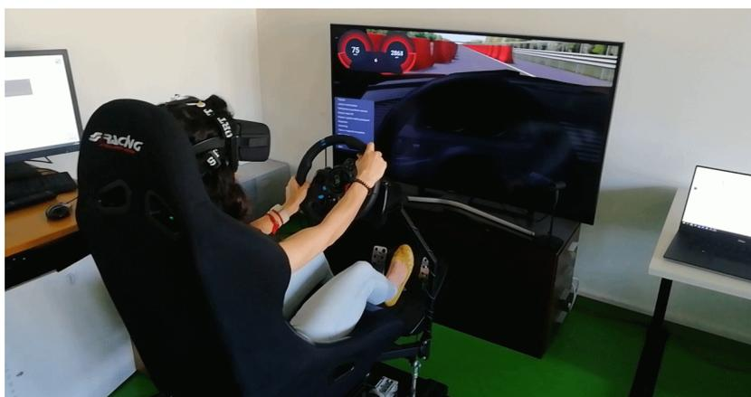
**Figure 5.** The driving simulator available in our laboratory at the University of Udine.
