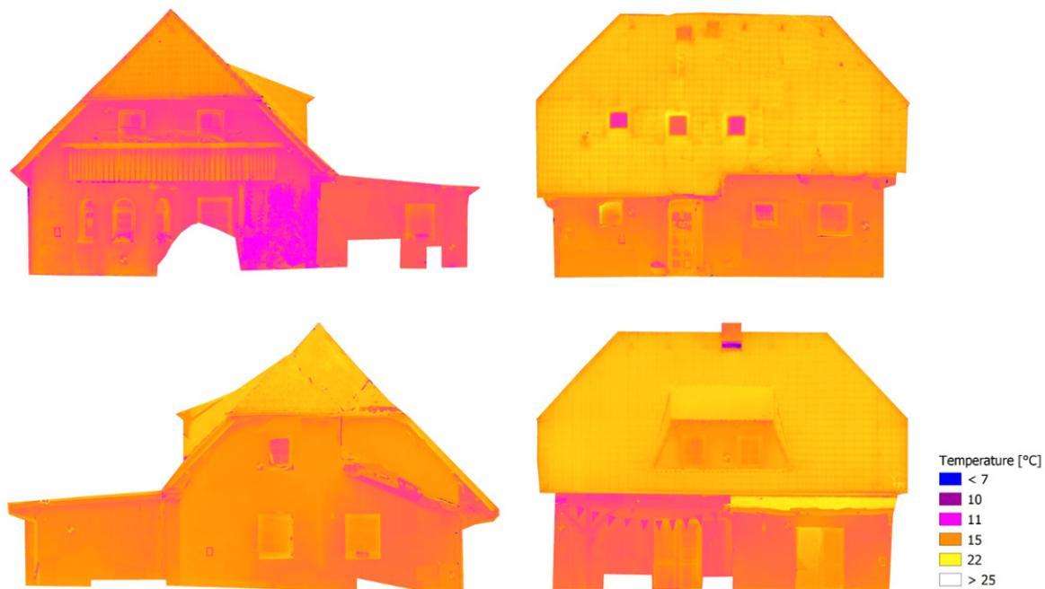
**Figure 10.** The resulting orthophotos augmented by thermal information.
