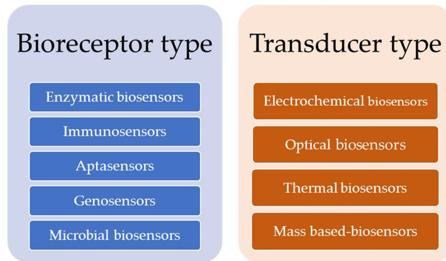
**Figure 2.** Classification of biosensors.
