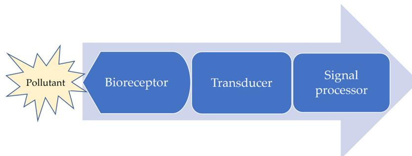
**Figure 1.** Operation of a biosensor.
