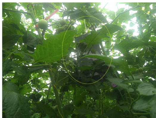
Figure 16. Sensors covered with plants can result in improper prediction due to the variation in RSSI.
