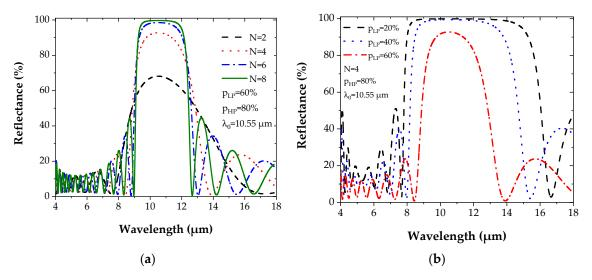
**Figure 4.** (a) The Bragg reflector for PGe materials with (a) porosities  $p_{LP} = 60\%$  and  $p_{HP} = 80\%$  while varying N. (b) Reflectance spectrum when N is fixed to 4, porosities  $p_{HP} = 80\%$ , and varying  $p_{LP}$ .
