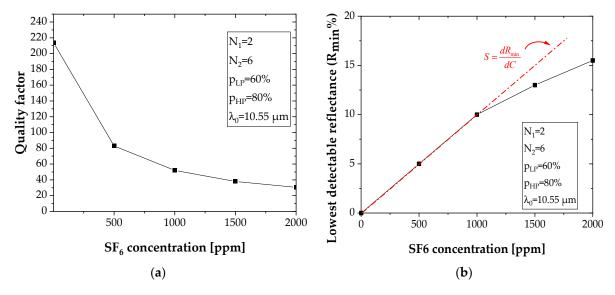
**Figure 9.** (a) Quality factor Q as a function of SF<sub>6</sub> concentration. (b) The lowest detectable reflectance as a function of concentration of target molecules.
