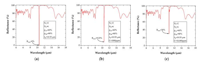
**Figure 8.** Reflectance spectrum of asymmetric microcavity, for PGe materials: without gas (**a**) and with SF<sub>6</sub> concentrations in air of (**b**) 1000 ppm, and (**c**) 10,000 ppm.
