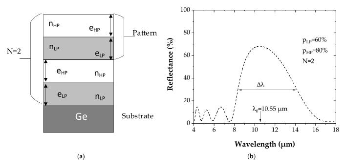
**Figure 2.** (a) Schematic of a PGe Bragg reflector made of a repeated pattern constituted by alternating a layer of low porosity (refractive index  $n_{LP}$  and thickness  $e_{LP}$ ) and a layer of high porosity (refractive index  $n_{HP}$  and thickness  $e_{HP}$ ). In this case, the pattern is repeated twice (N = 2). (b) Calculated reflectance spectrum of the corresponding PGe Bragg reflector, with values of 60% and 80% for the low and the high porosities, respectively.
