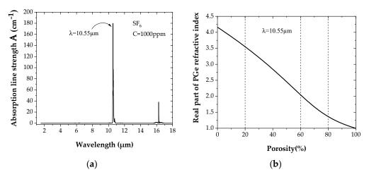
**Figure 1.** (a) Mid-IR absorbance spectrum of SF<sub>6</sub> (for a SF<sub>6</sub> concentration of 1000 ppm in air). (b) Dependence of the real part of the PGe refractive index on porosity.
