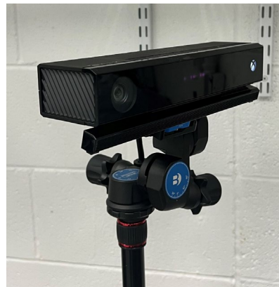
Figure 6. Kinect v2 ToF sensor mounted to a tripod using a 3-way geared head.
