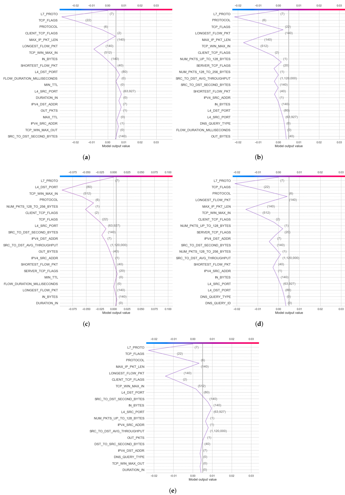
Figure 15. Decision plot results of local explanation for NF-BoT-IoT-v2 dataset in five Cat output values: (a) 0—DoS; (b) 1—DDoS; (c) 2—Reconnaissance; (d) 3—Benign; (e) 4—Thref.
