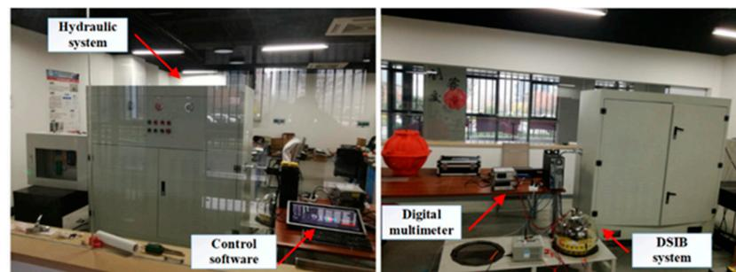
**Figure 14.** Hardware-in-the-loop system experimental platform: mainly includes hydraulic device, simulation control software, digital multimeter, and DSIB system.
