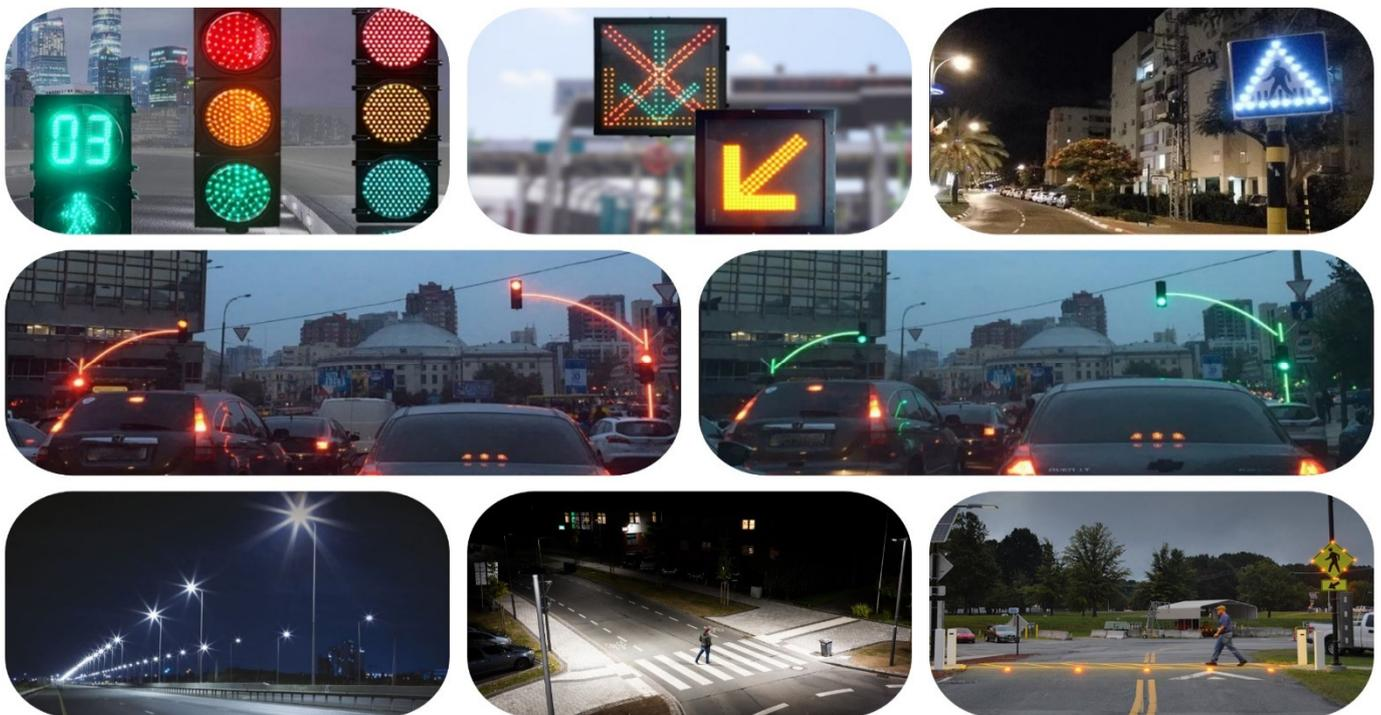
**Figure 1.** LED lighting sources installed in road and pedestrian infrastructures, capable of providing communications through visible light and optical camera communications.
