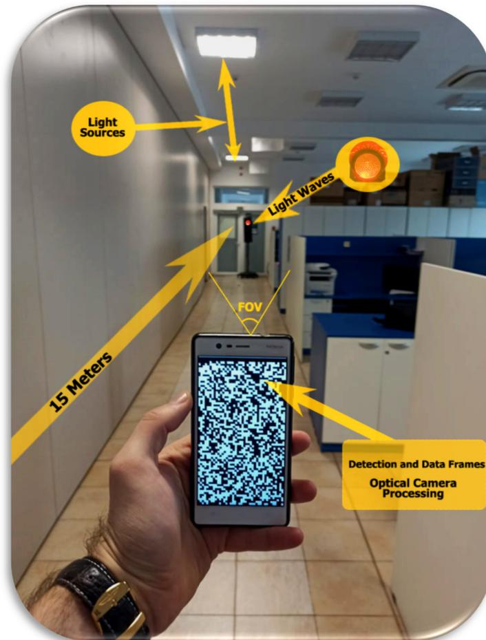
**Figure 10.** Detection process in an indoor scenario with disturbing lighting sources over a distance of 15 m.
