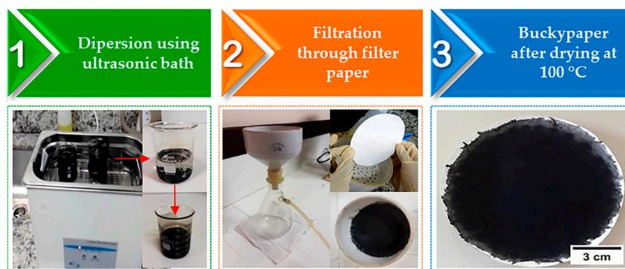
**Figure 1.** Schematic flowchart of BP production steps. (1) Dispersion; (2) filtration; (3) final buckypaper element.
