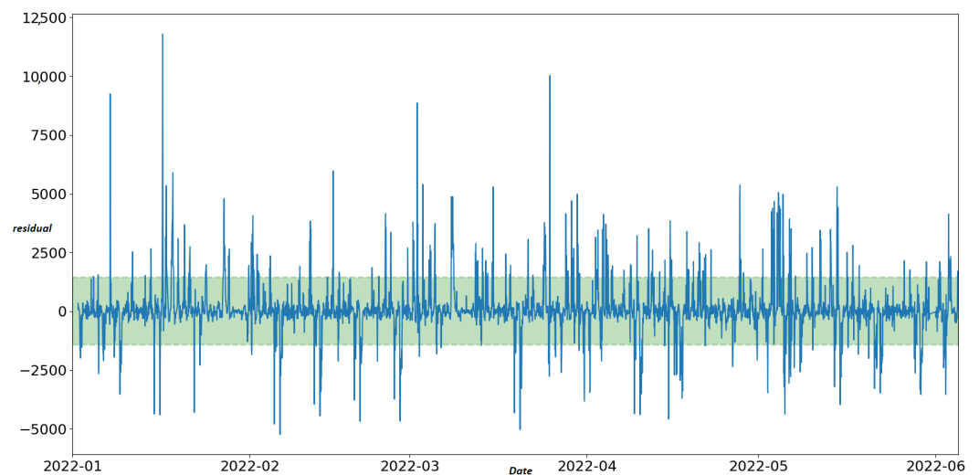
Figure 5. Residual curve of sensor “MS734” with the upper and lower fences of the IQR method. The green dots represent unusual traffic conditions. Red dots represent sensor faults.
