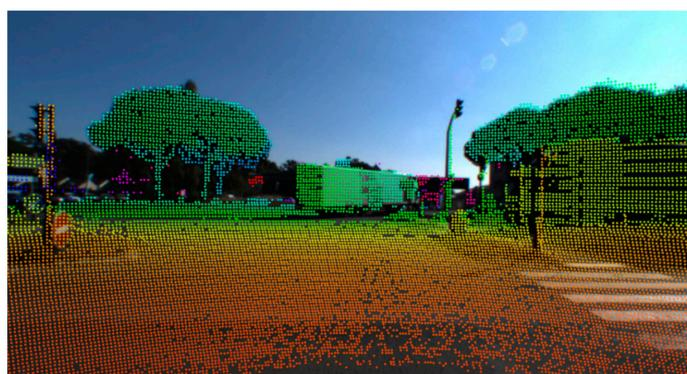
Figure 6. Lidar point cloud projected onto camera images.
