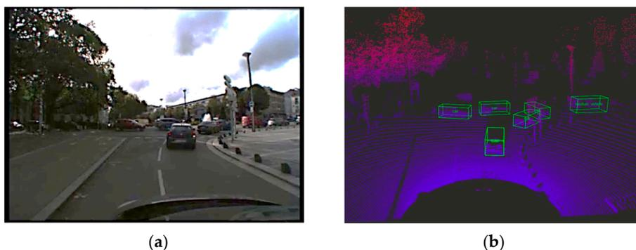
**Figure 9.** Object detection by DCNN: (a) camera image for illustration and (b) result of lidar DCNN detection.
