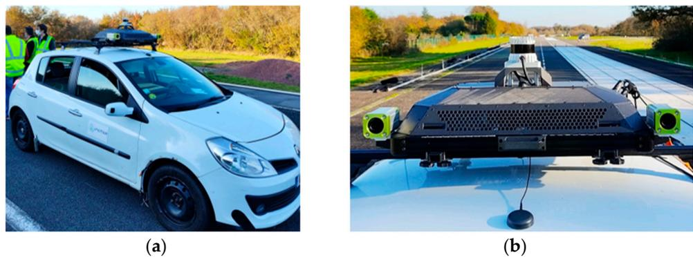
**Figure 2.** (a) Perception and localization system installed on an experimental vehicle; (b) zoom of the PLS.
