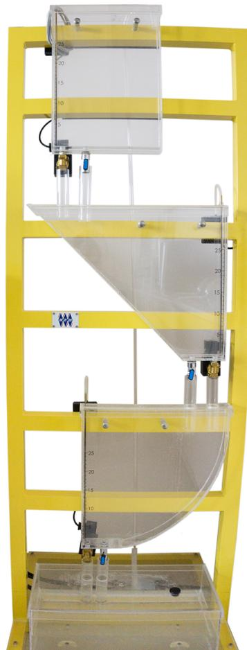
**Figure 1.** The laboratory multi-tank system.
