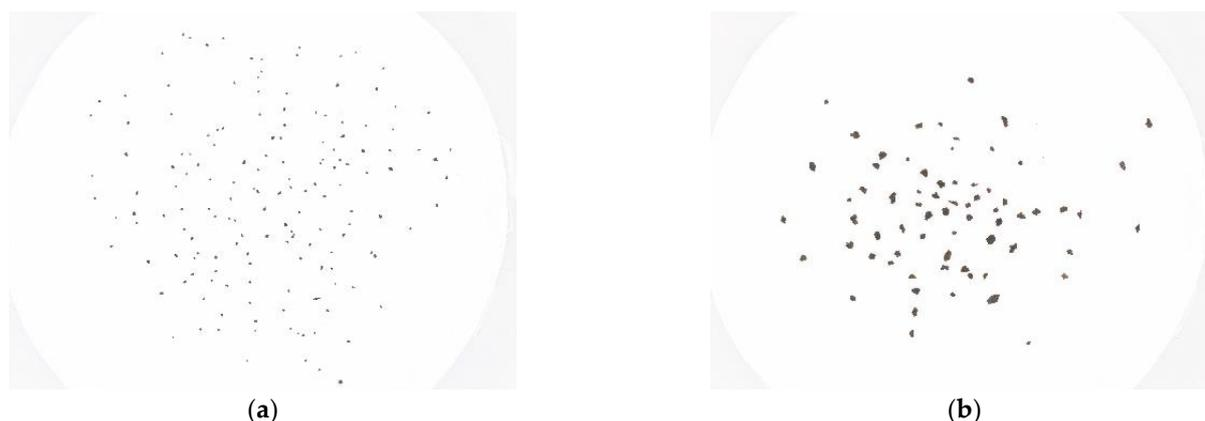
**Figure 10.** Pictures acquired by the vision system using four samples of real volcanic ash particles: (a) granulometry class G1, (b) G2.
