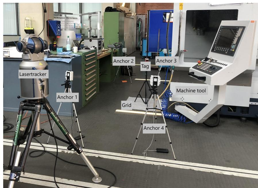
**Figure 3.** Setup with laser tracker.
