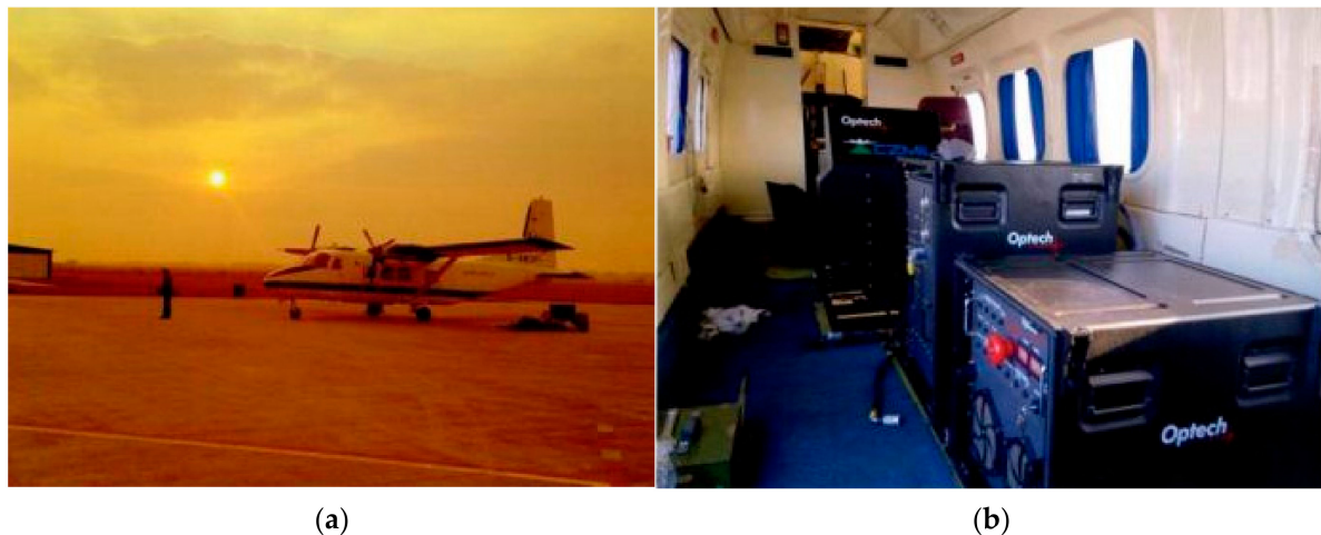
Figure 2. ALB system used in the experiment: (a) Y-12 aircraft, (b) Optech CZMIL.
