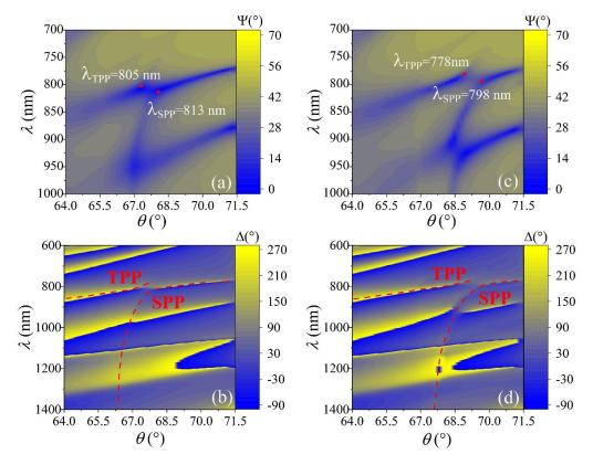
**Figure 3.** The dispersion maps  $\lambda$  ( $\theta$ ) of ellipsometric parameters  $\Psi$ (°) (**a**,**c**) and  $\Delta$ (°) (**b**,**d**) for structure PC (TiO<sub>2</sub>/SiO<sub>2</sub> (110 nm/200 nm)/with gold nano-bumps (50 nm) in water (left side) and in ethanol (right side). The red points show the strong coupling effect between the Tamm plasmons and the surface plasmon at zero detuning.
