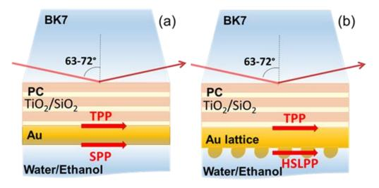
**Figure 1.** Scheme of excitation configurations of the PC(TiO<sub>2</sub>/SiO<sub>2</sub>)/Au structures for generating the TPP-SPP (**a**) and TPP-HSLPP (**b**) modes by spectroscopic ellipsometry in total internal reflection (TIR).
