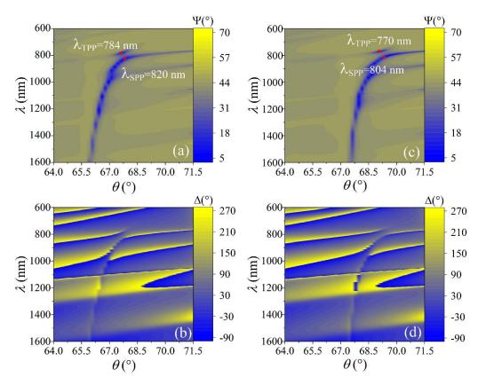
**Figure 2.** The dispersion maps  $\lambda$  ( $\theta$ ) of ellipsometric parameters  $\Psi$ ( $^{\circ}$ ) (**a**,**c**) and  $\Delta$ ( $^{\circ}$ ) (**b**,**d**) for structure PC (TiO<sub>2</sub>/SiO<sub>2</sub> (110 nm/200 nm)/Au (50 nm) in water (left side) and in ethanol (right side). The red points show the strong coupling effect between the Tamm plasmons and the surface plasmon at zero detuning.
