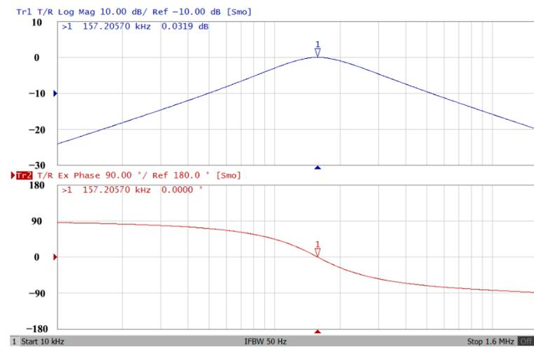
**Figure 30.** Frequency-domain characteristics of the measured amplitude and phase responses of the first proposed circuit at  $V_{O1}$ .
