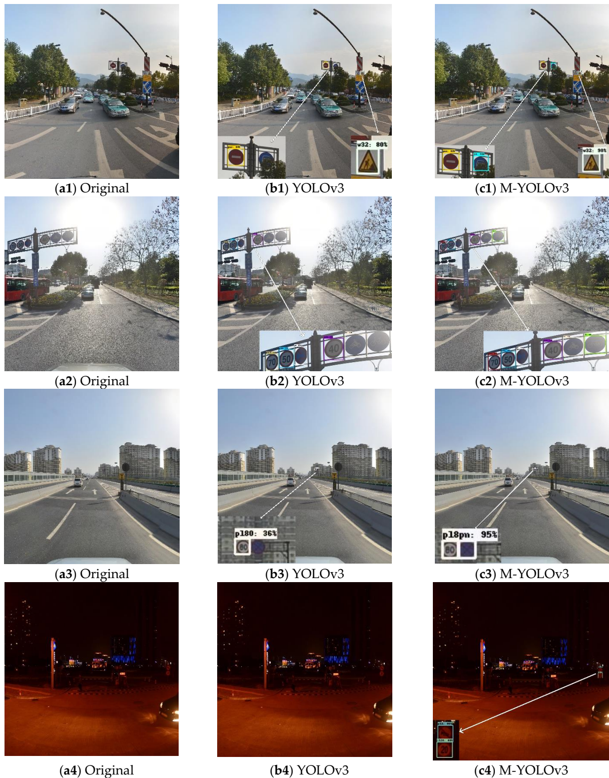
Figure 14. Comparison of the recognition effect of traffic signs under special environments.
