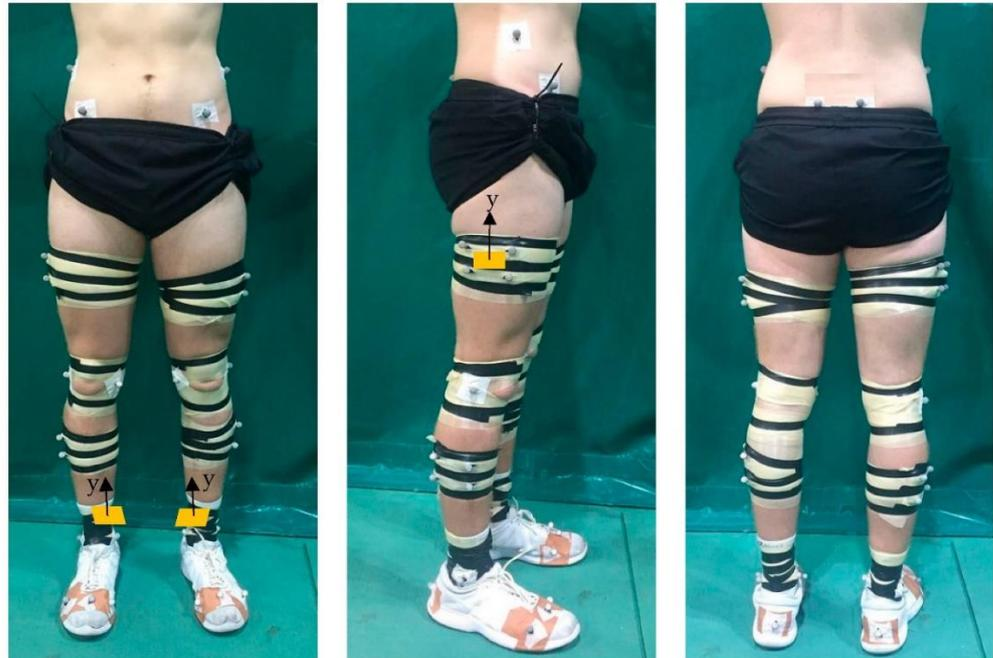
**Figure 1.** Example marker and IMU set up. Orange rectangles represent location of IMUs. IMU: inertial measurement unit.
