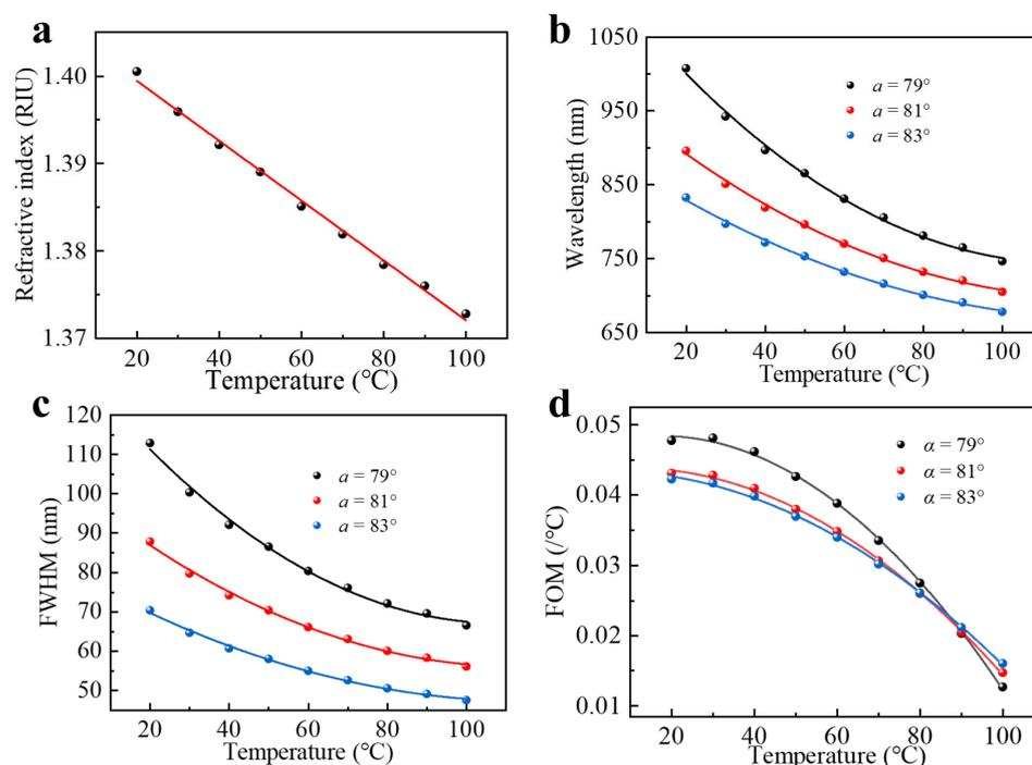
**Figure 2.** (a) Variation of RI of n-butanol with temperature. (b) Simulated SPR wavelengths. (c) Spectral FWHM and (d) spectral FOM as a function of temperature under different fiber polishing angles. The nonlinear fitting curves are to guide the eyes.
