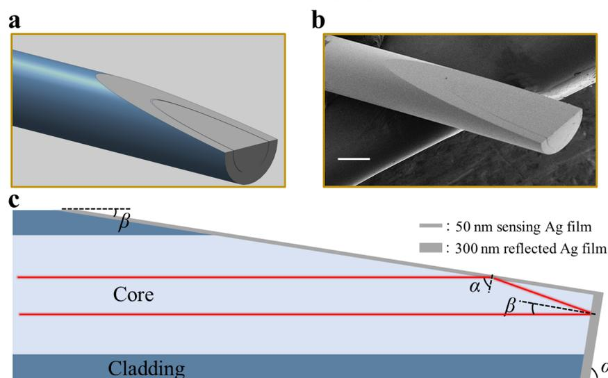
**Figure 1.** (a) Schematic view of the wedged fiber optic SPR probe. (b) Scanning electron microscope image of the fabricated probe. Scalebar:  $200 \mu\text{m}$ . (c) Definition of involved parameters of the sensing probe.
