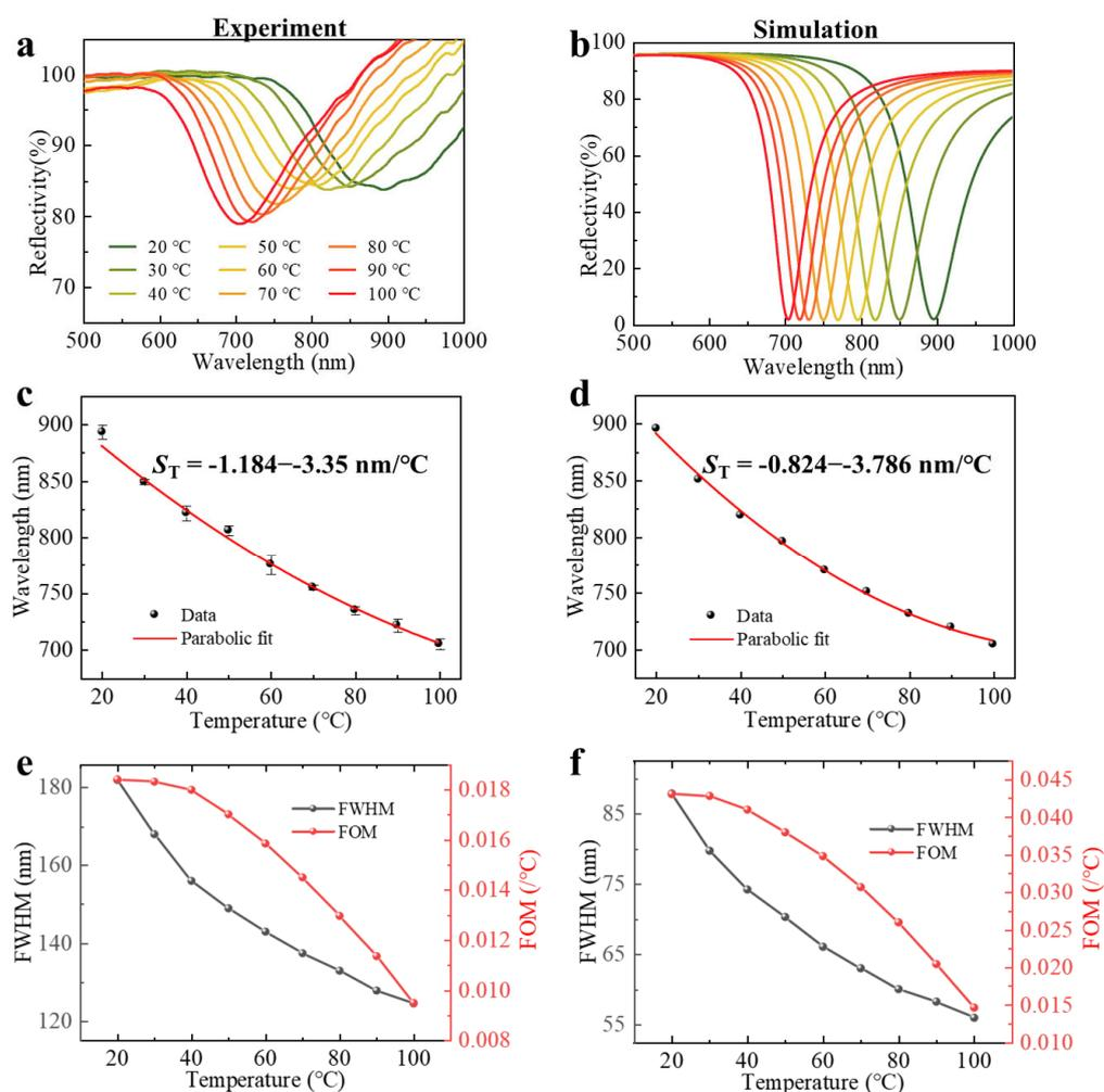
**Figure 5.** (a) Experimental and (b) simulated reflection spectra for different temperatures. (c,d) Resonance wavelengths as a function of temperatures, which correspond with panels (a) and (b), respectively. (e) Experimental and (f) simulated spectral FWHM and FOM change with temperature.
