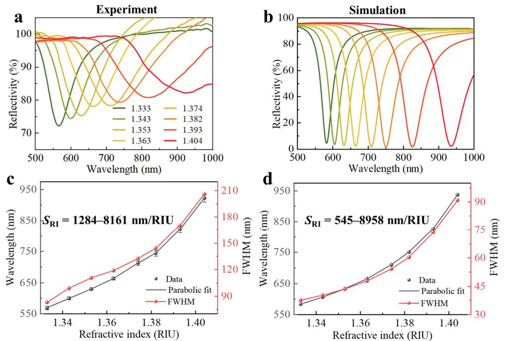
**Figure 4.** (a) Experimental and (b) simulated reflection spectra for different RIs. (c,d) Resonance wavelengths and spectral FWHM as a function of RIs, which correspond with panels (a) and (b), respectively.
