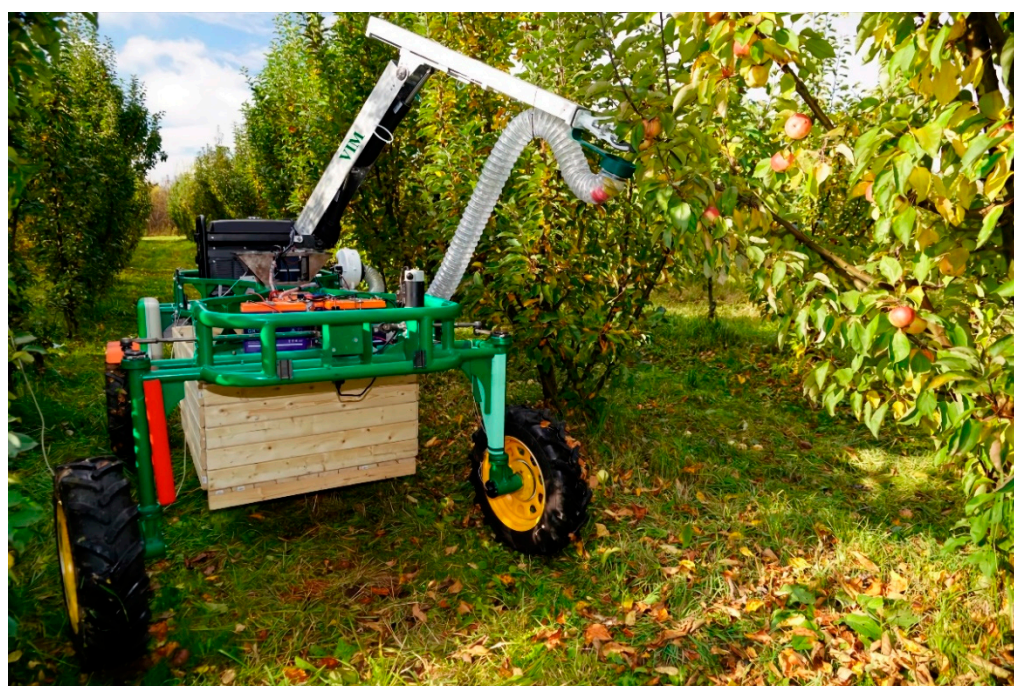
Figure 2. Wheeled robotic platform with a robotic device for fruit removal.
