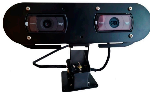
Figure 6. Stereo camera of the apple fruit identification system.
