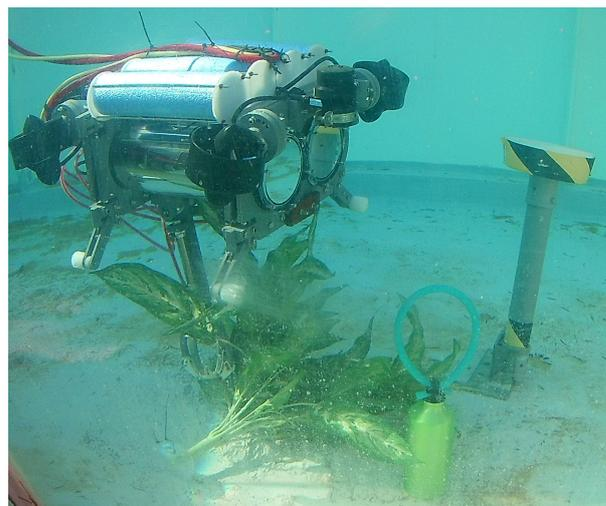
**Figure 1.** The *UDrobot* picking up a plant in an underwater environment.
