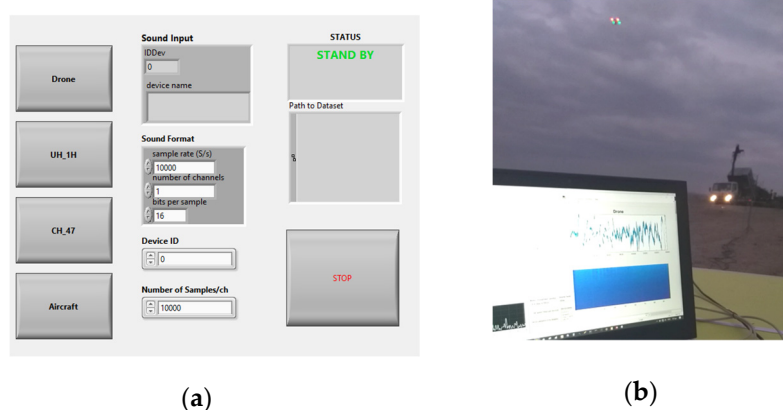
Figure 11. Application interfaces for (a) audio sample collection for CNN training and (b) identification of targets. Notice how the system detects the UAS's presence, even when a heavy crane truck is working in the vicinity.
