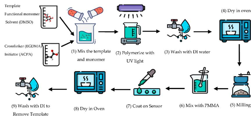
**Figure 6.** Illustration preparation of the sensor.
