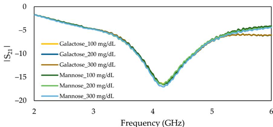
**Figure 15.** Measured frequency response of the insertion loss ( $S_{21}$ ) of main MIP-coated microwave-based stub biosensor exposed to mannose and galactose solutions ranging from 100 mg/dL to 300 mg/dL.
