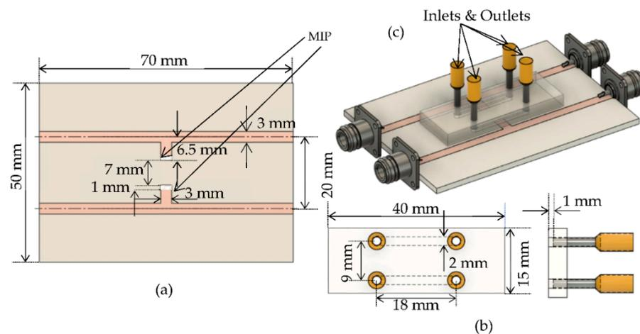
**Figure 2.** The designed MIP-coated microwave-based stub biosensor (a) Top view of the biosensor (b) Top view and side view of the microfluidic system with the inlets and outlets (c) View of the assembled biosensor.
