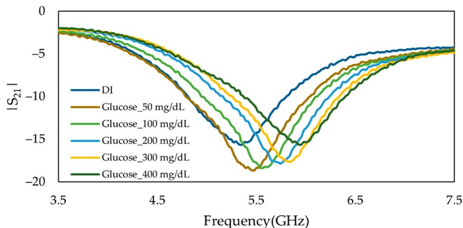
**Figure 11.** Measured frequency response of the insertion loss ( $S_{21}$ ) of duplicate MIP-coated microwave-based stub biosensor for the glucose solutions with concentration ranging from 50 mg/dL to 400 mg/dL.
