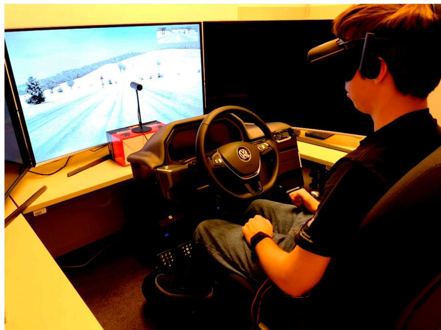
**Figure 1.** Illustration of the Nervtech driving simulator interior. Image is distributed under the Creative Commons Attribution License and taken from the study by Gruden et al. [4].
