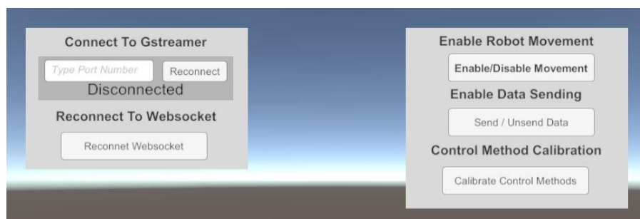
Figure 7. The graphical user interface of our system connects with Gstreamer and WebSocket server (robot control software), allows enabling/disabling the robot's movements or sending data, and for starting the calibration process of the control methods.
