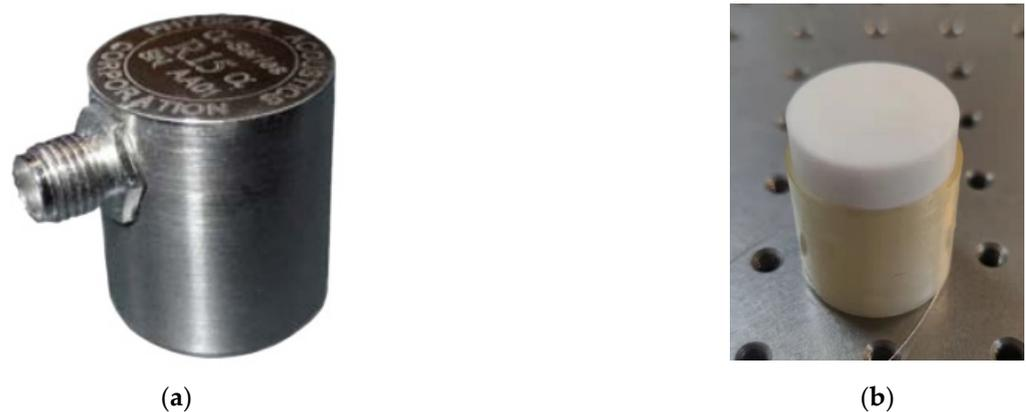
Figure 9. (a) Sound source PZT; (b) optical fiber ultrasonic sensor.
