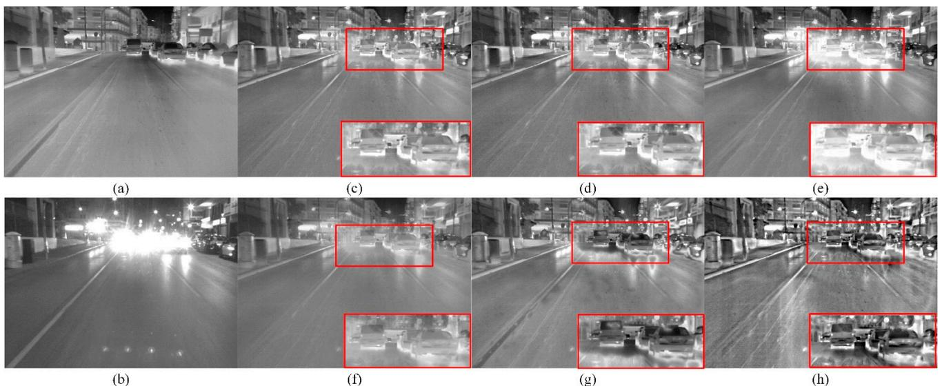
**Figure 1.** Fused images in the glare scene using six different methods. (a) Infrared image; (b) Visible image; (c) MDLatLRR; (d) MGFF; (e) MSID; (f) ResNet; (g) RGFF; (h) Proposed.
