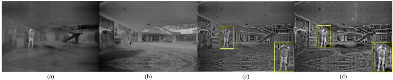
**Figure 11.** Test result in the smoke scene. (a) Infrared image; (b) Visible image; (c) Fused image on FPGA; (d) Fused image on PC.
