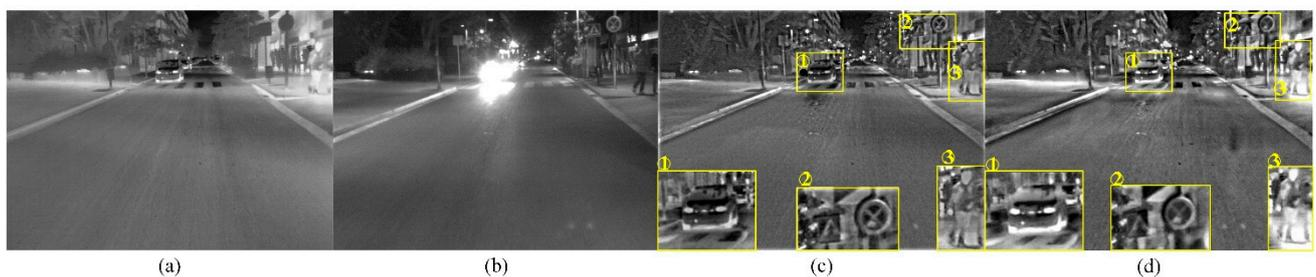
**Figure 10.** Test result in the glare scene. (a) Infrared image; (b) Visible image; (c) Fused image on FPGA; (d) Fused image on PC.
