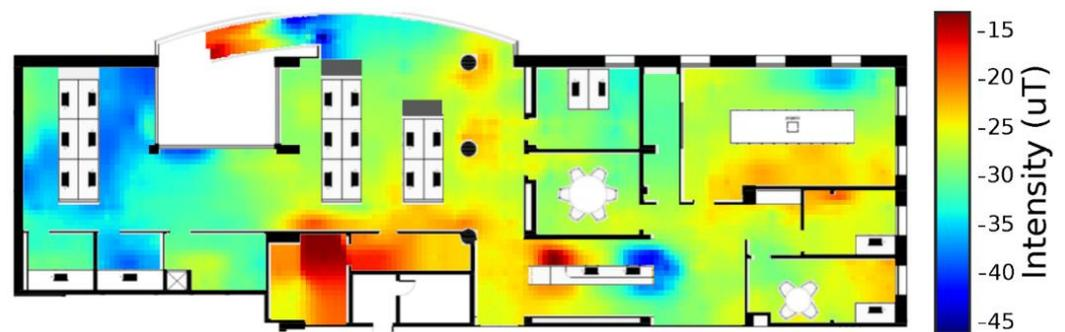
**Figure 3.** Plan of a building used to test an algorithm for the construction of the magnetic fingerprint. The vertical bar on the right represents the magnetic field intensity. In the floor plan, colour intensity correlates with people activity. Data were collected from six people walking with their smartphones and the walking paths were then acquired (reproduced under the terms and conditions of the Creative Commons Attribution (CC BY) license from [70]).
