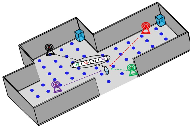
**Figure 1.** The working process of Wi-Fi fingerprinting indoor localization. A comparison of collected fingerprints in the database helps to estimate the locations of different clients (reproduced under the terms and conditions of the Creative Commons Attribution (CC BY) license from [43]).
