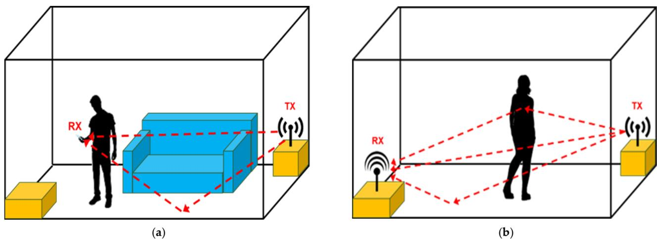
**Figure 4.** (a). Device-based approach. (b). Device-free approach. Effect of human presence on multipath environment. An RF signal propagates from the transmitter to the receiver via multiple paths, i.e., multipath components. The presence and position of people furtherly affect the multipath environment, while people motion introduces signal frequency shifts, i.e., Doppler effect.
