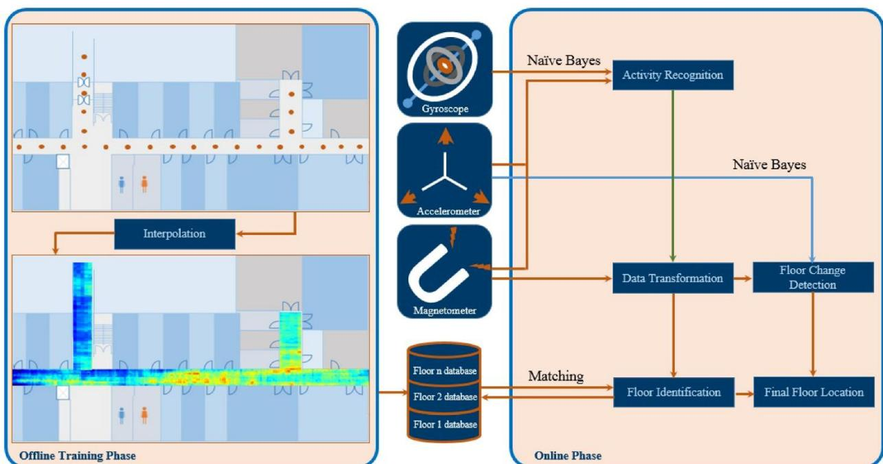
**Figure 6.** A three-step model for Floor Identification based on magnetic field data captured with smartphone sensors. (reproduced under the terms and conditions of the Creative Commons Attribution (CC BY) license from [5]).
