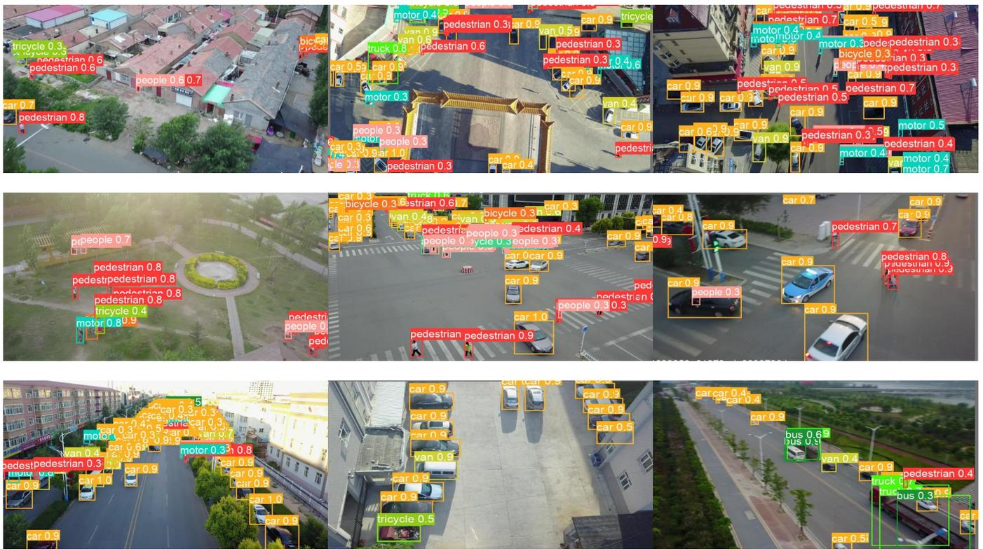
**Figure 8.** Visualization of some of the output of our suggested architecture on some of the test images of the VisDrone 2021 dataset.
