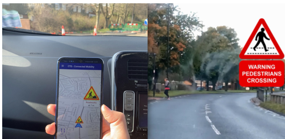
Figure 1. Examples of C-Mobile C-ITS services—the RWW system ( left , Road Work Warning—informs drivers in a timely manner about road works, restrictions, and instructions) and the concept WSP system ( right , Warning System for Pedestrians, detects risky situations, e.g., road crossing, involving pedestrians, allowing the possibility to warn vehicle drivers).
