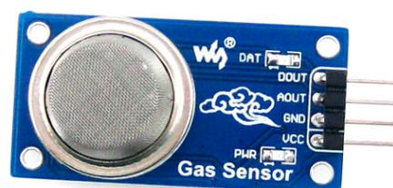
Figure 2. MQ2 Gas Sensor.
