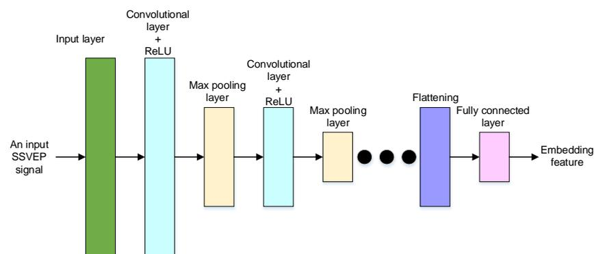
**Figure 3.** The neural network structure of the embedding feature encoder.
