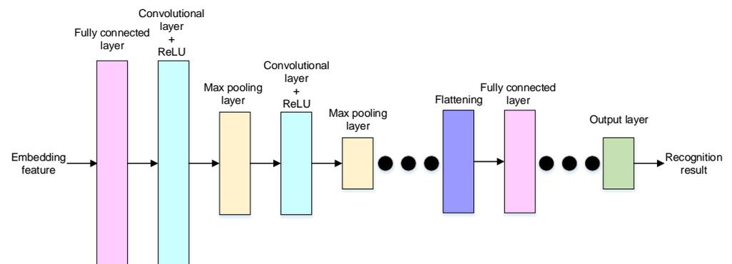
**Figure 5.** The neural network structure of the classification decoder.
