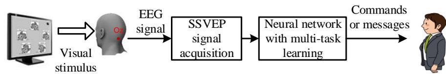
**Figure 1.** The flowchart of the proposed SSVEP-based BCI with MTL includes a visual stimulation procedure, SSVEP signal acquisition, and neural network with MTL.
