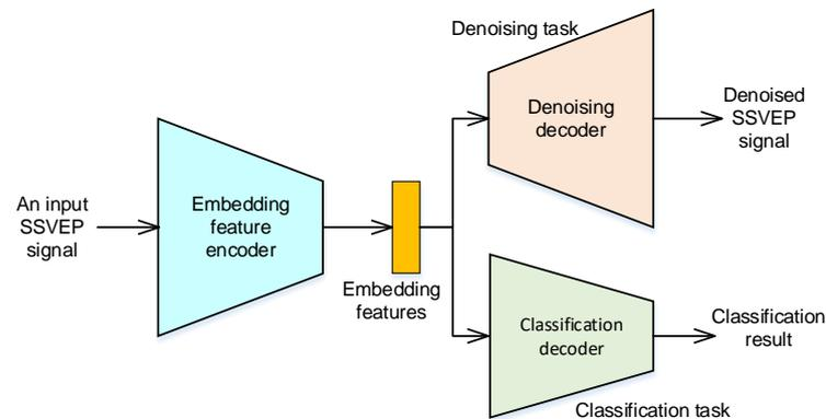
**Figure 2.** The framework of the proposed multi-task based neural network.
