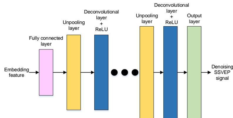
**Figure 4.** The neural network structure of the denoising decoder.
