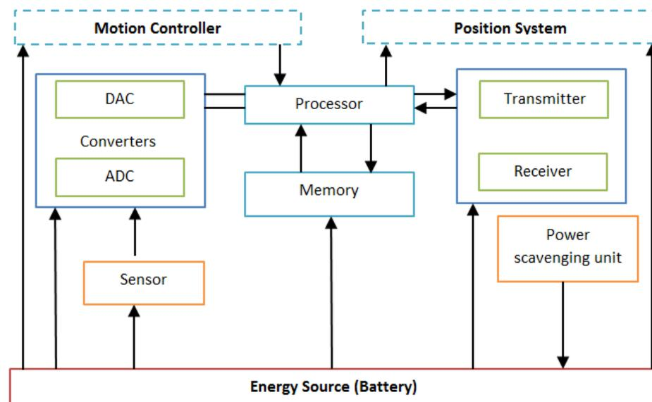
**Figure 5.** Generic sensor node structure.
