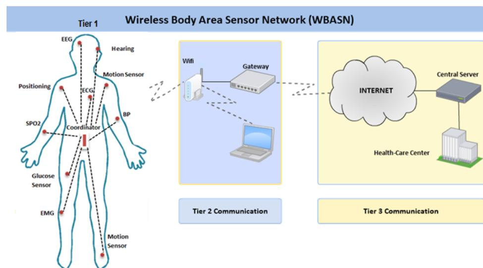
**Figure 1.** Wireless body area sensor network overview.
